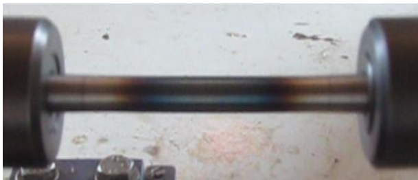
Fig. 4 Burning effect of CHS at maximum bending moment Fig. 5 Crack initiation and nature of failure
