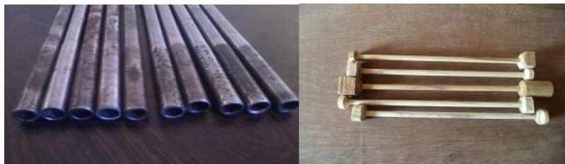
Fig. 1 Semi finished specimens of CHS and teak wood
