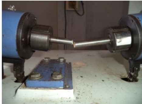
Fig. 6 Fatigue failure of WFCHS
