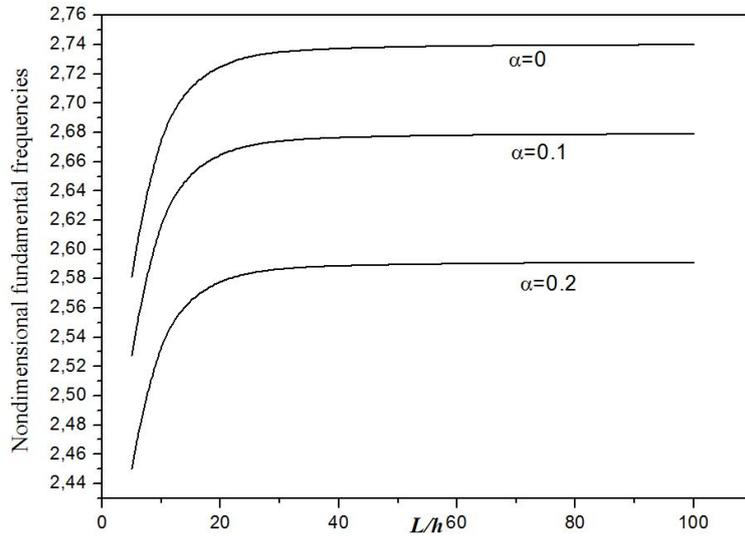
Fig. 3 Variation of the fundamental frequency  $\left( \bar{\omega} = (\omega L^2 / h) \sqrt{I_0 / \int_{-h/2}^{h/2} E(z) dz} \right)$  of FG beams ( $k = 1$ )
