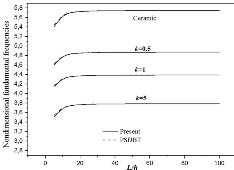
Fig. 2 Variation of the fundamental frequency  $(\bar{\omega} = (\omega L^2 / h) (\rho_M / E_M))$  of FG beams with  $L / h$  ratio for various values of the power-law exponent
