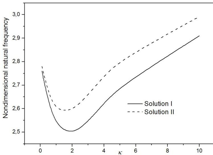
Fig. 5 Variation of the fundamental frequency  $\left( \bar{\omega} = (\omega L^2 / h) \sqrt{I_0 / \int_{-h/2}^{h/2} E(z) dz} \right)$  of imperfect FG
