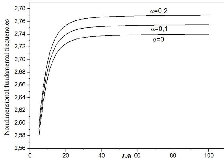
Fig. 4 Variation of the fundamental frequency  $\left( \bar{\omega} = (\omega L^2 / h) \sqrt{I_0 / \int_{-h/2}^{h/2} E(z) dz} \right)$  of FG beams ( $k = 1$ )
