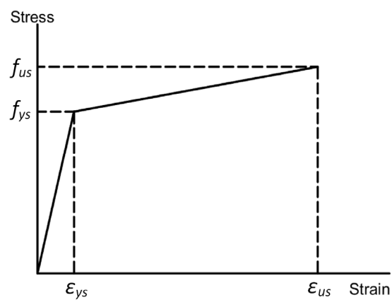
Fig. 4 Stress-strain diagram of the steel
