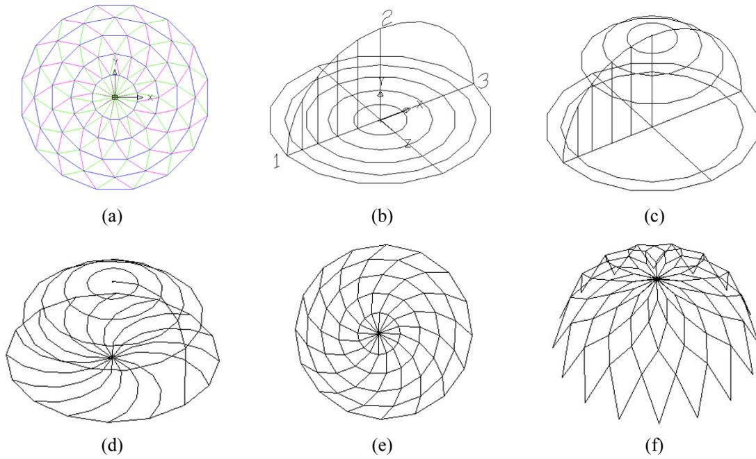
Fig. 3 Foldable dome extended from the two-dimensional structure
