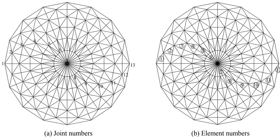
Fig. 9 The design model of the hybrid barrel vault with typical node and element numbers
