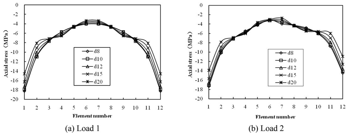
Fig. 17 Influence of the cable cross section area on the axial stress of steel bars
