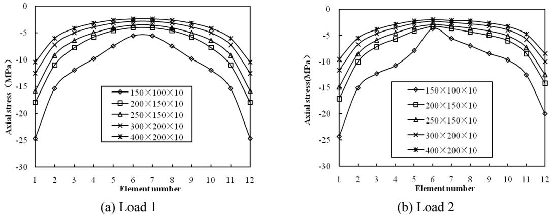
Fig. 15 Influence of steel bar cross section area on its axial stress
