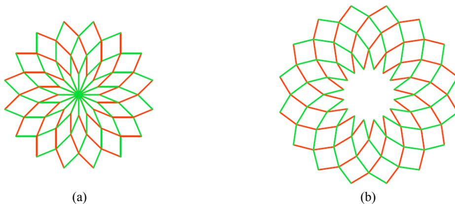
Fig. 2 Foldable bar structures
