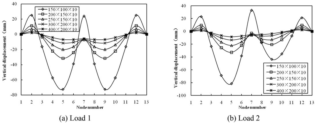
Fig. 14 Influence of steel bar cross section area on the nodal displacement
