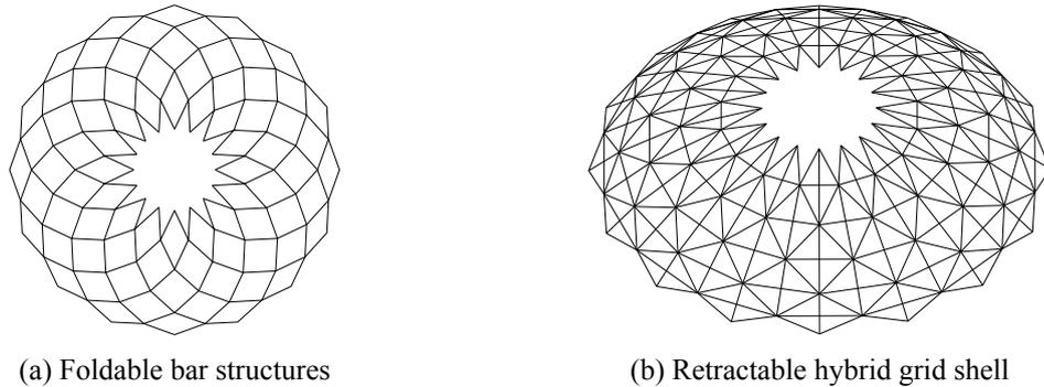
Fig. 6 Deployment state of the system
