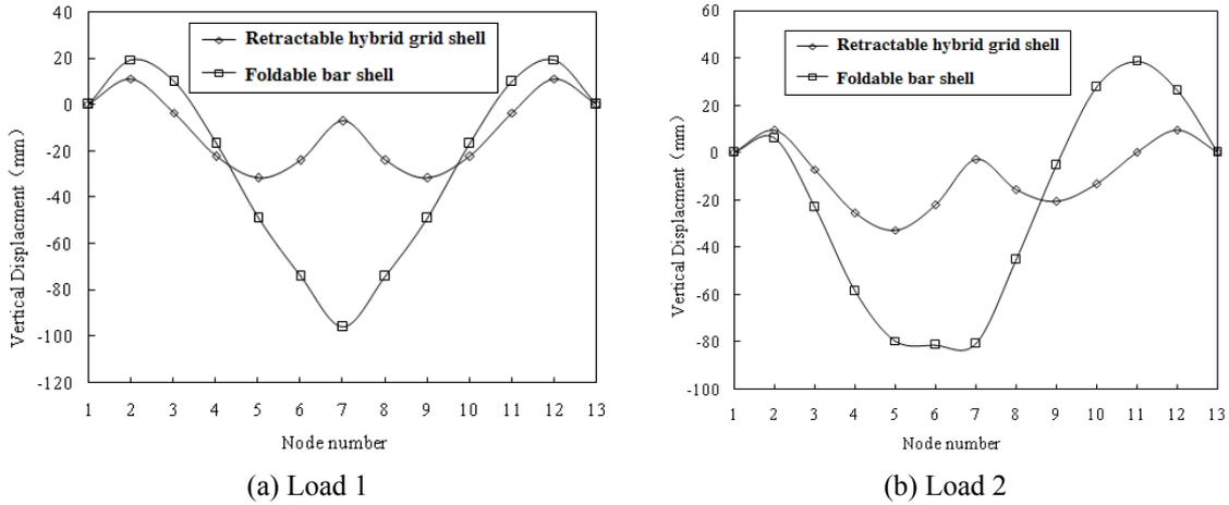
Fig. 10 Nodal displacements of the foldable bar structure and retractable hybrid grid shell
