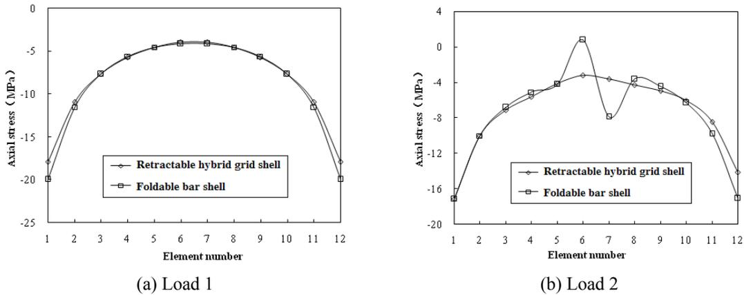
Fig. 11 Steel bar axial stresses of the foldable bar structures and retractable hybrid grid shell
