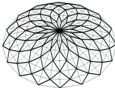
Fig. 7 3D hybrid grid shell model
