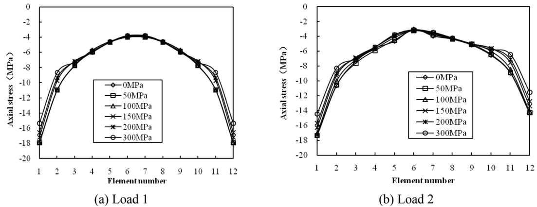
Fig. 19 Influence of the initial prestress on the axial stress of steel bars
