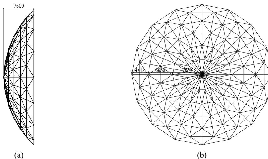
Fig. 8 Geometric parameters of the hybrid grid shell (mm)
