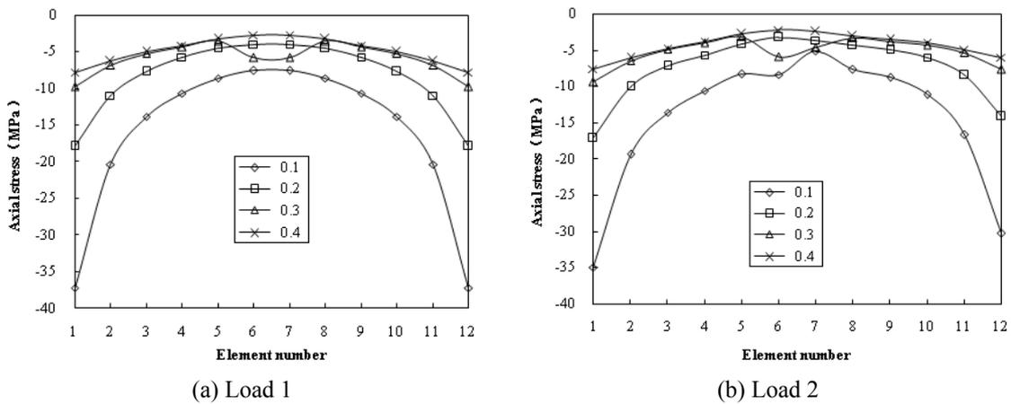
Fig. 13 Influence of rise-span ratios on the axial stress of steel bars
