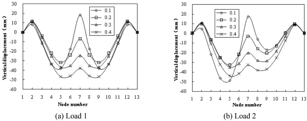
Fig. 12 Influence of rise-span ratios on the nodal displacement
