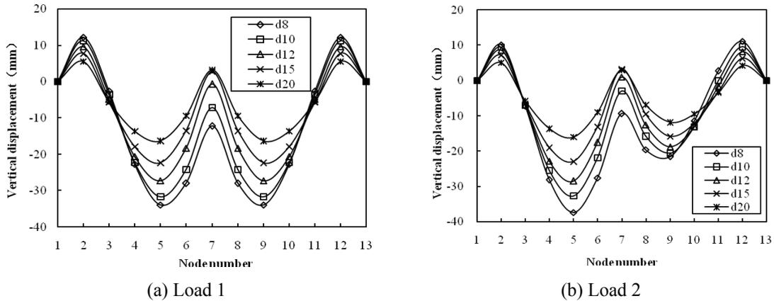
Fig. 16 Influence of the cable cross section area on the nodal displacement
