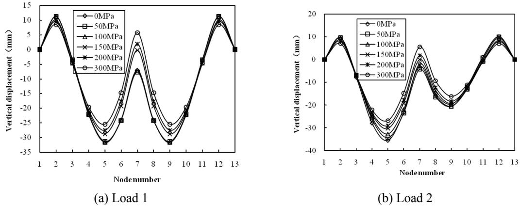
Fig. 18 Influence of the cable initial prestress on the nodal displacement
