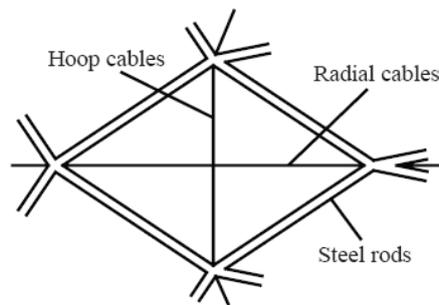
Fig. 4 Radially retractable hybrid grid shell
