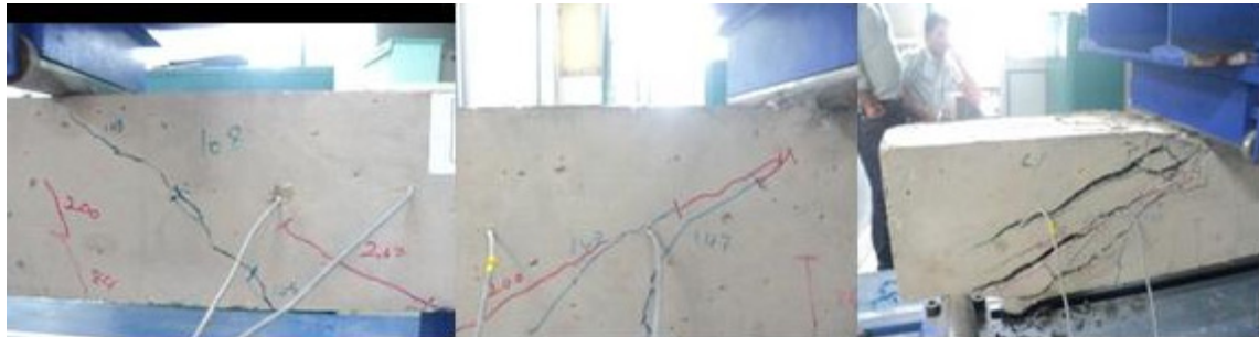
Fig. 12 Failure mode of beam C_{16} -D-2-2
