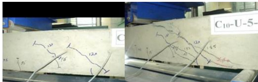
Fig. 14 Failure mode of beam C_{10} -U-5-2
