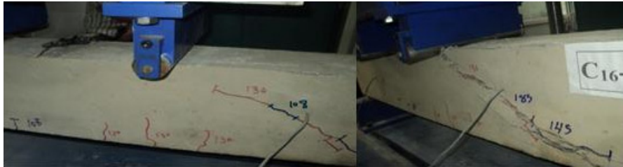
Fig. 11 Failure of beam C_{16-D-2-1}
