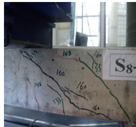
Fig. 8 Failure mode of beam S 8 -1
