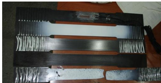
Fig. 4 Specimen with front surface with random speckle patterns (on top) and back surface (bottom) with strain gage installed
