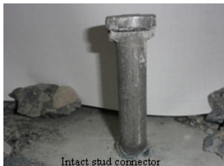
(c) Intact stud connector
