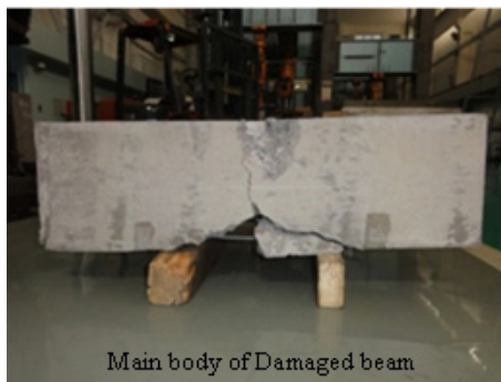
(a) Main body of damaged beam
