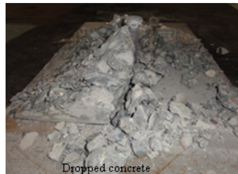
(b) Dropped concrete from damaged beam
