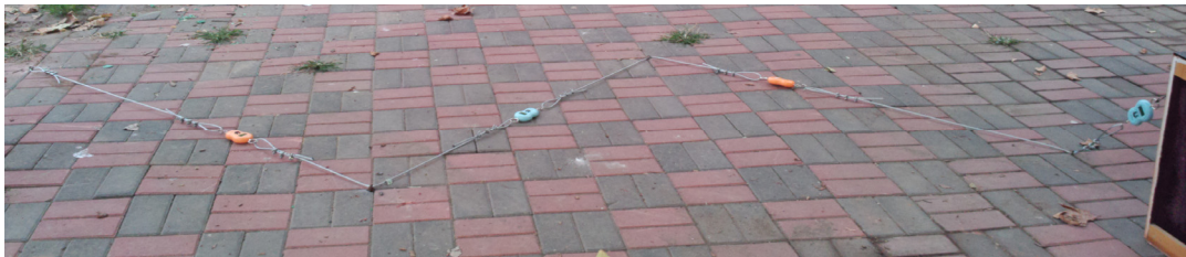
Fig. 12 Continuous sliding cable in the test
