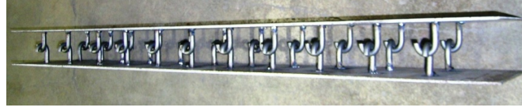
(a) SCS sandwich beam with J-hook connectors
