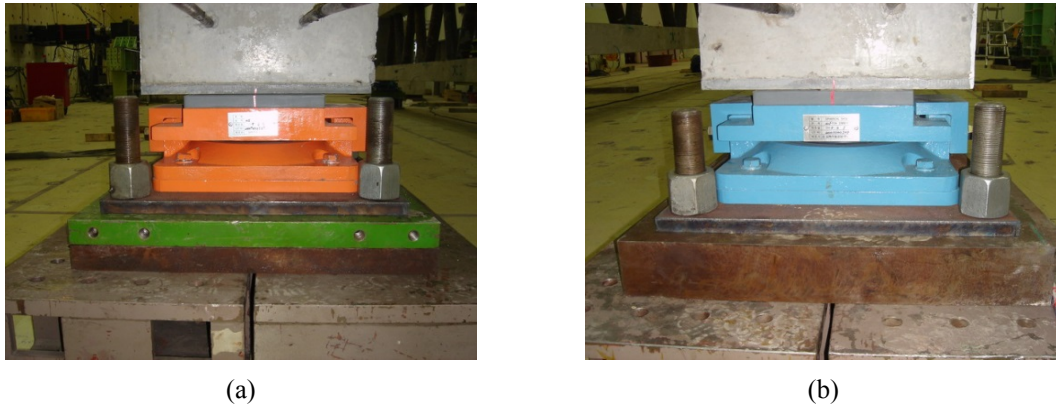
Fig. 3 Details of end supports: (a) spherical bearing (hinge); and (b) spherical bearing (roller)
