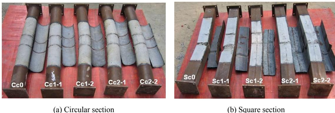
Fig. 5 Typical failure pattern of core concrete
