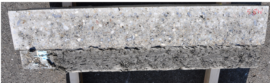
Fig. 15 Concrete block after diamond cutting. Cement grout remains attached to rough concrete. Specimen PR100_5
