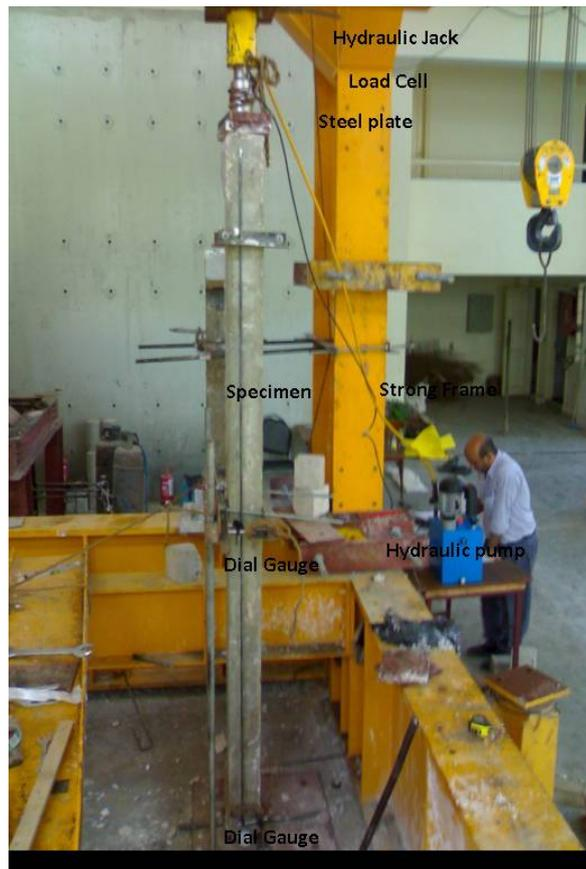
Fig. 3 Typical test setup for specimens
