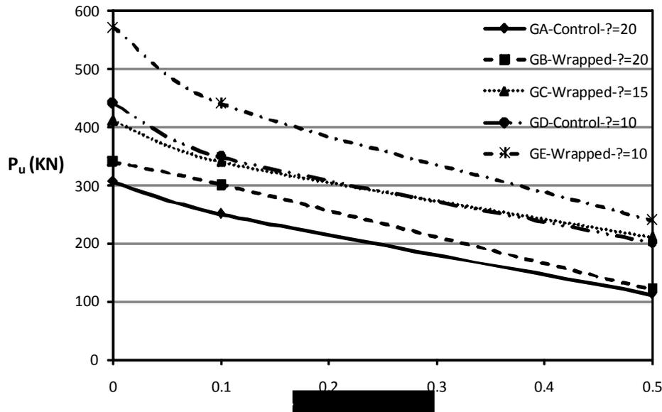
Fig. 4 Effect of confinement on ultimate load
