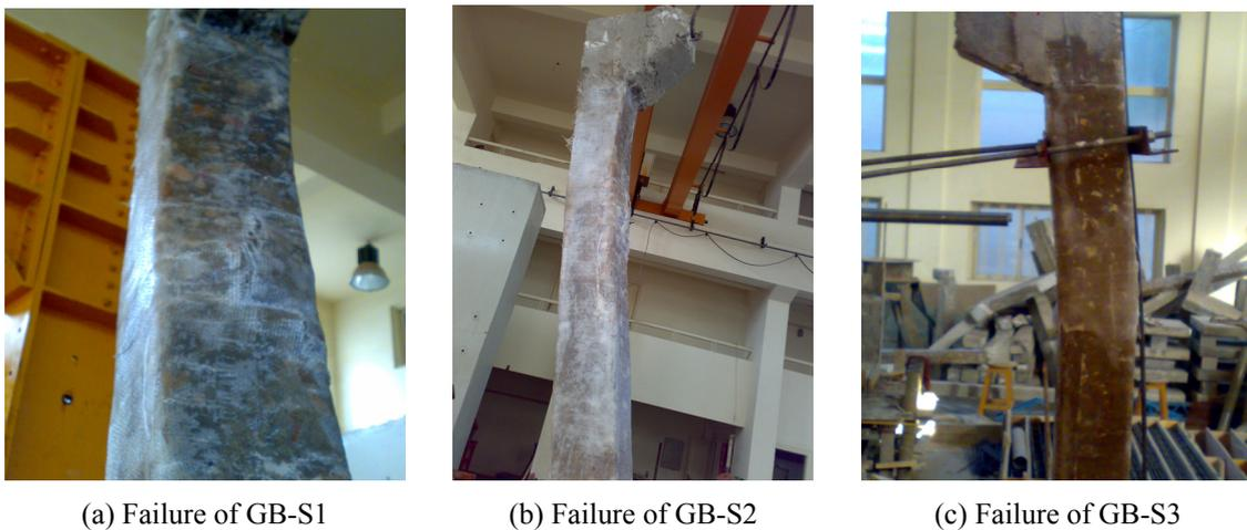
Fig. 8 Failure patterns of wrapped slender columns
