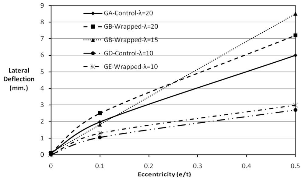
Fig. 6 Effect of confinement on lateral deflection at failure
