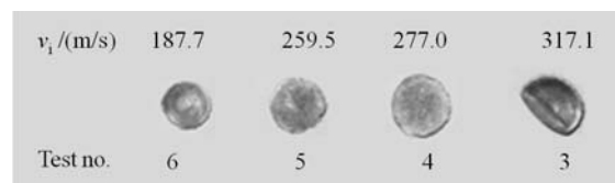
Fig. 6 Some plugs collected after tests
