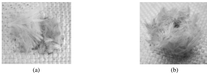
Fig. 7 Damage view of FRP laminate for test no. 11: (a) front view; and (b) rear view
