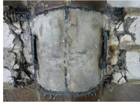
Fig. 9 Concrete of joint zone after testing
