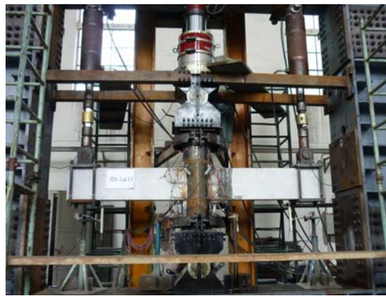
Fig. 7 Experimental setup for cyclic tests of side column specimens
