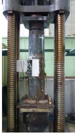
Fig. 3 Experimental setup for axial compression test
