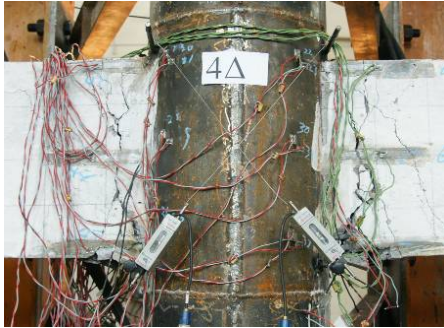
Fig. 8 Bending failure at beam end
