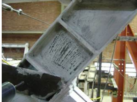
Fig. 3 Yielding of the second panel at 10th cycle of lateral loading
