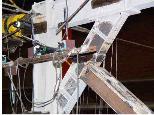
Fig. 5 Termination of KBF1 test by fracture of knee-diagonal brace weld at KBF1 test specimen
