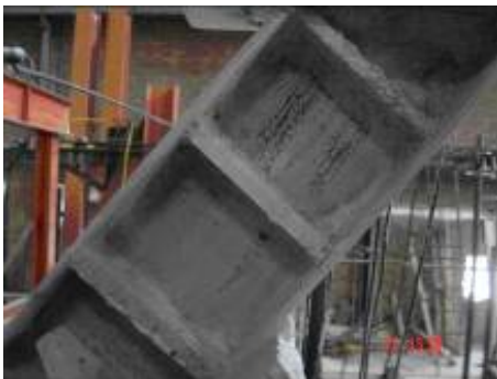
(a) Yielding of the second panel at 7th cycle of loading
