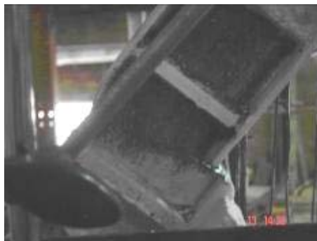
(c) Tearing on the web of knee element at third panel
