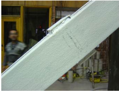
(a) Local yielding of diagonal brace at 18.9 mm lateral displacement
