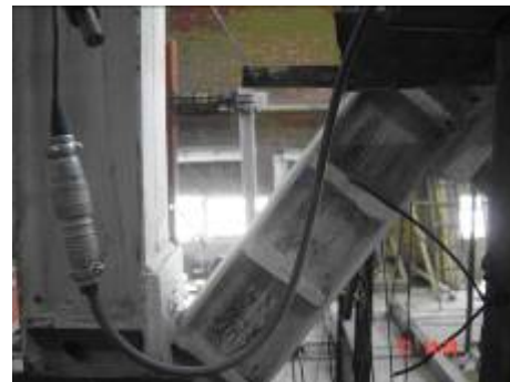
(b) Yielding of the 5th and 7th panels at 11th cycle of loading
