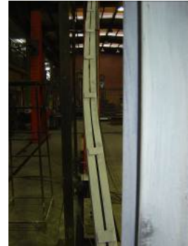
(b) Overall buckling of diagonal brace at 22.3 mm lateral displacement
