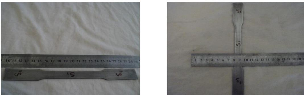
Fig. 3 Final shape of steel plate
