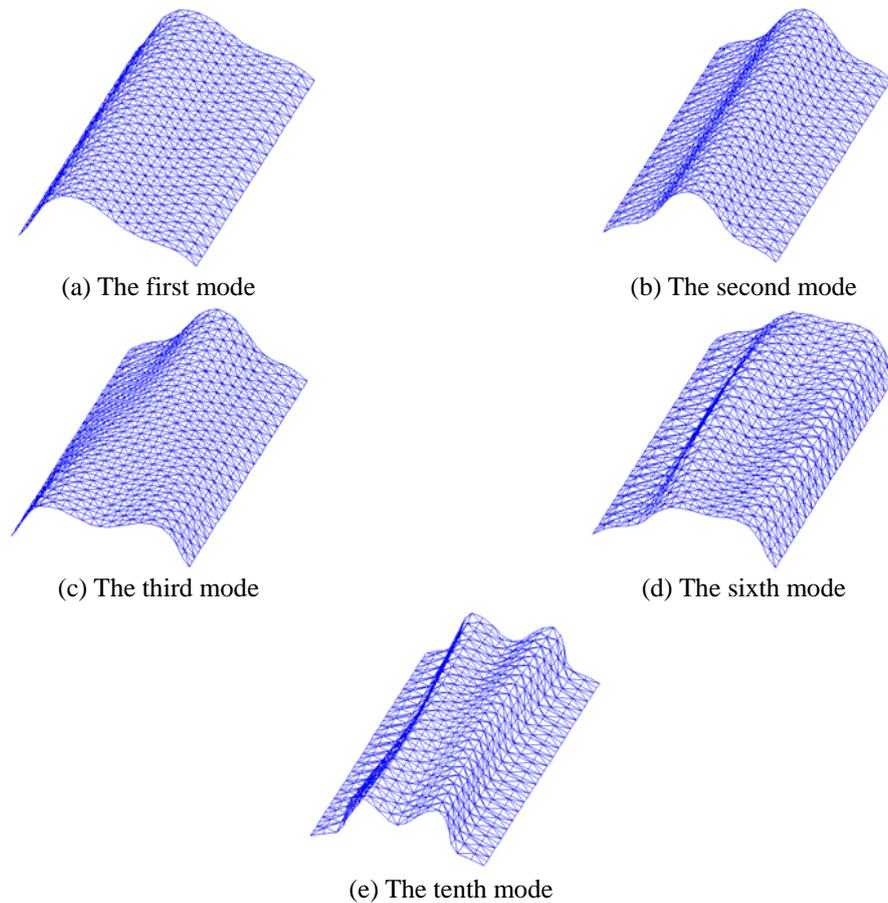
Fig. 3 Buckling modes of the hybrid barrel vault
