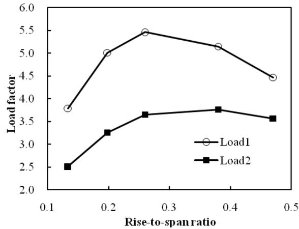
Fig. 12 Failure loads with different rise-to-span ratios
