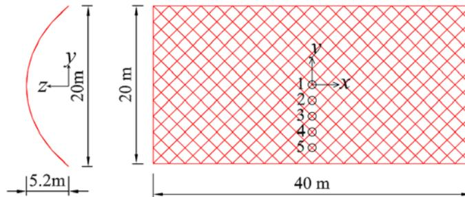
Fig. 2 The design model of the hybrid barrel vault with typical nodes and element numbers
