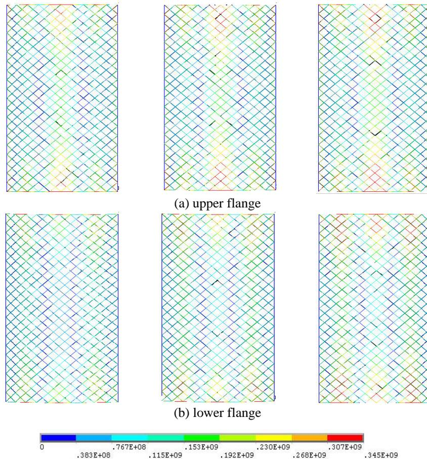
Fig. 7 The development process of the plastic zone (Pa)
