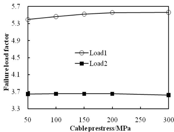
Fig. 15 Failure loads with different cable pre-stress
