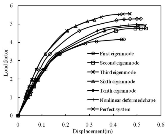
Fig. 9 Load-displacement curves for imperfect structures, loading case  $g+s$
