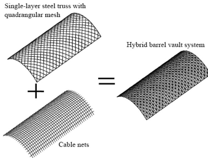
Fig. 1 The hybrid barrel vault system
