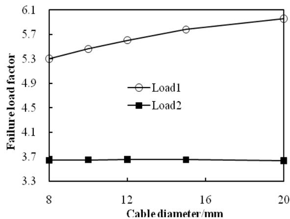
Fig. 14 Failure loads with different areas of cables
