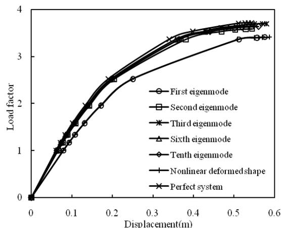
Fig. 10 Load-displacement curves for imperfect structures, loading case  $g+s/2$
