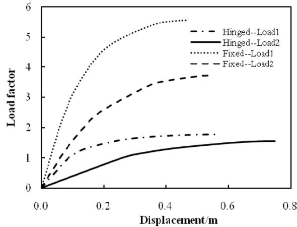
Fig. 16 Load–deflection curves of the hybrid structure with different support conditions
