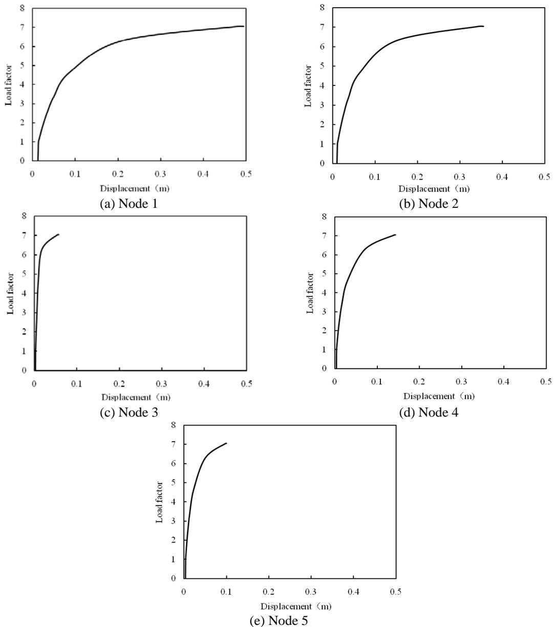
Fig. 4 Load factor vs. displacement for geometrical non-linear buckling analysis
