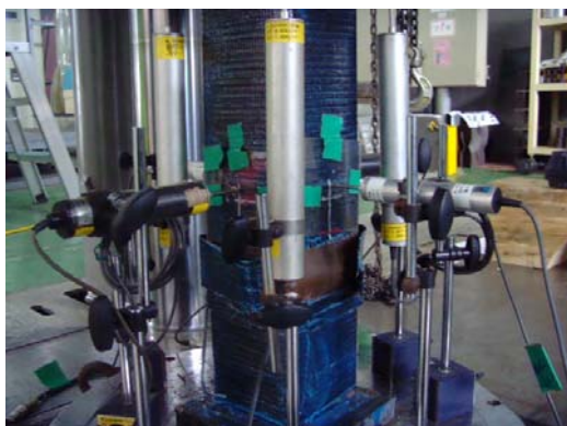
(c) FRP rupture (R6F-3, Axial displacement = 10 mm)
