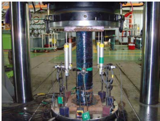
(a) FRP rupture (C4F-1, Axial displacement = 7.1 mm)
