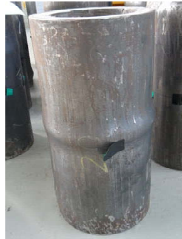
(b) Symmetric buckling in the mid-height(No.20)
