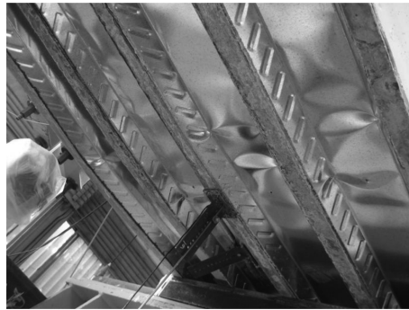
Fig. 10 Buckling at the compression side of the steel sheet for tested specimen
