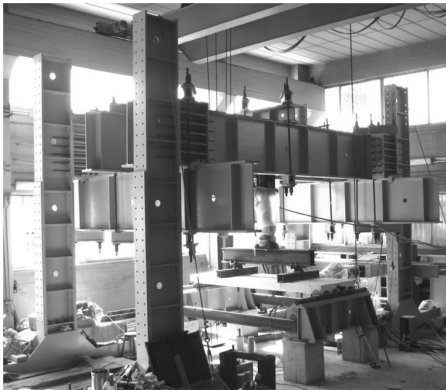
Fig. 4 Experimental set-up with specimen CPLL in place
