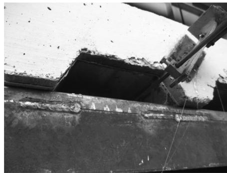
Fig. 9 End slip of specimen CPLL1
