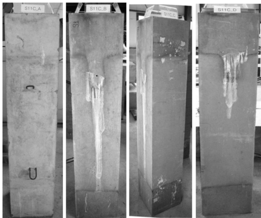
Fig. 9 Spalling of S11C after fire test
