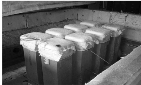
Fig. 5 Photo of a fire testing furnace with short columns
