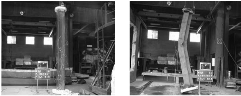
Fig. 8 Test column before and after fire test of H-section
