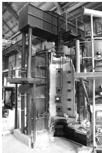
Fig. 6 Testing equipment for column fire tests
