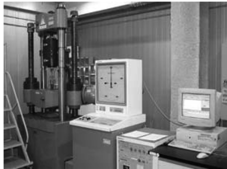
Fig. 2 Testing machine for tensile coupon tests at high temperatures
