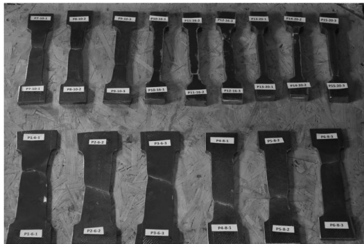
Fig. 5 Tested coupons after tensile test ( t = 6, 8, 20, 15, 10 mm, starting from bottom left counterclockwise)
