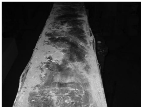
Fig. 8 Local buckling of steel plates in the compression zone of beams
