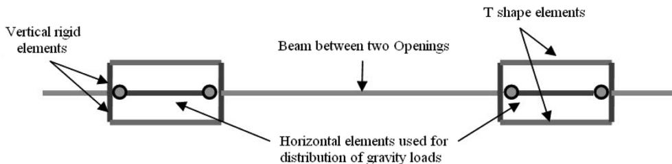
Fig. 2. The simplified model of a beam with two web openings
