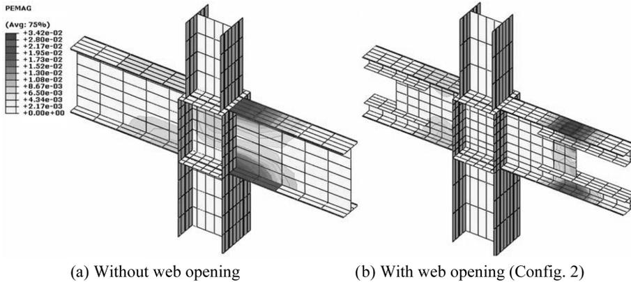
Fig. 8. Distribution of plastic strain at middle connection of first story (drift 4%)
