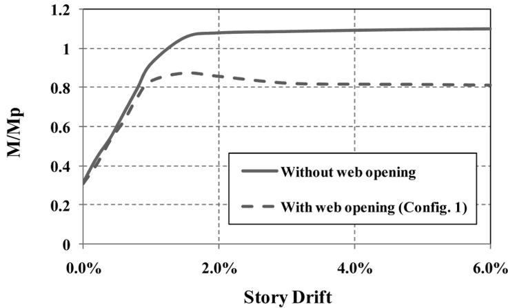
Fig. 9. Effect of web openings on reduction of  $M/M_p$
