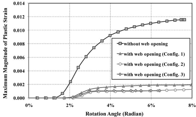
Fig. 7. Maximum plastic strain at panel zone area versus roof rotation angel
