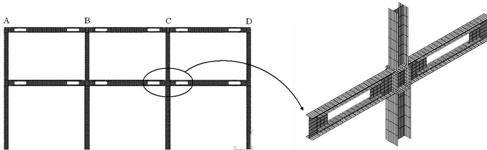
Fig. 5. Finite model of reference structures with web openings
