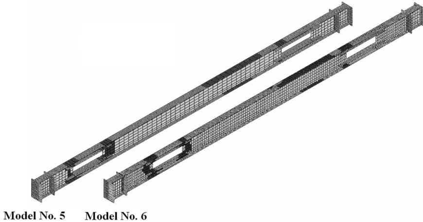
Fig. 4. Distribution of yielded elements in beams with openings at two ends (drift 2%)
