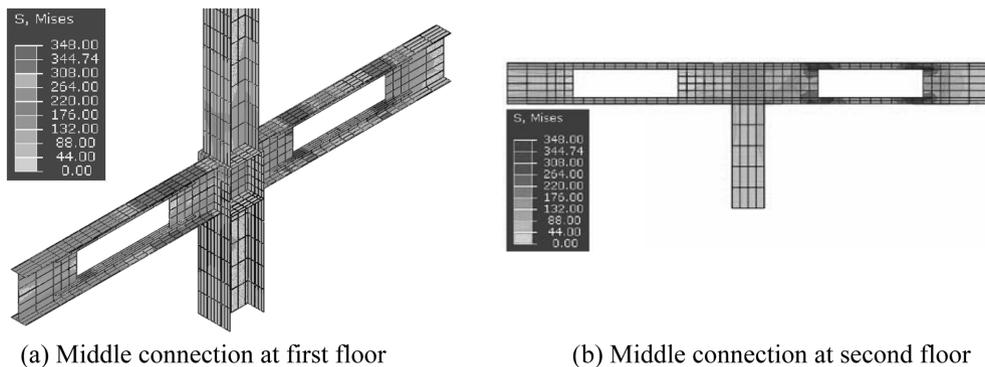
Fig. 11. Stress distribution at connection area for model TF236PRH (drift 2%)
