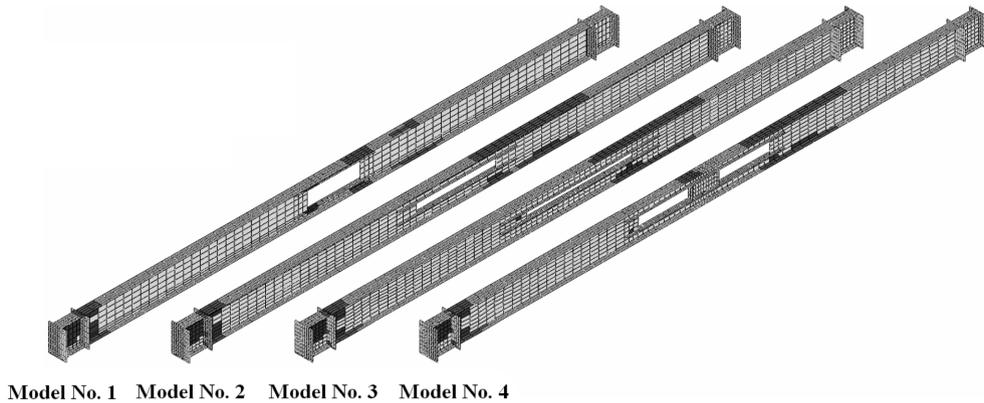
Fig. 3. Distribution of yielded elements in beams with openings at mid-span (drift 2%)
