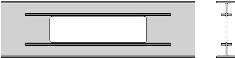
Fig. 1. A typical opening in the beam web
