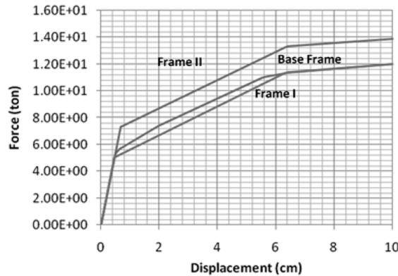
Fig. 8 Compression between model's push over analysis results
