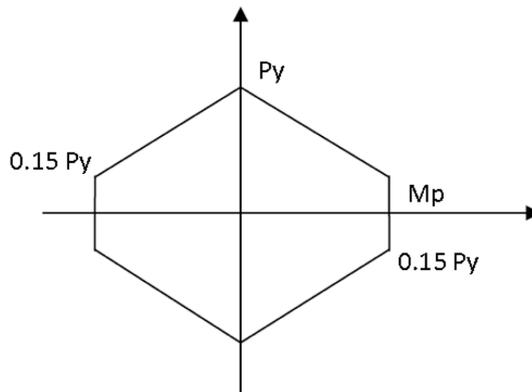
Fig. 5 Yield interaction surface for the beam-column elements
