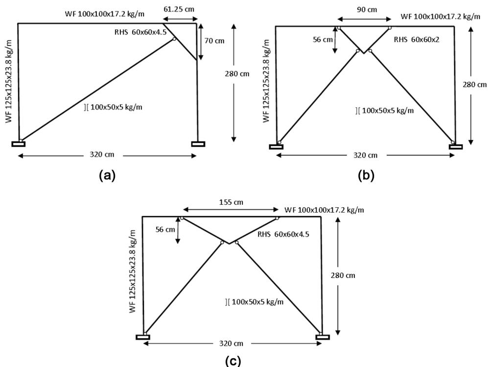
Fig. 6 Base frame, Frame I and II dimensions and section properties (a) Base frame (b) Frame I (c) Frame II
