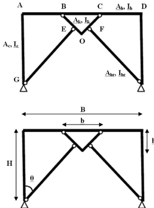
Fig. 1 General form of Hat Knee Bracing system (*HKB*)
