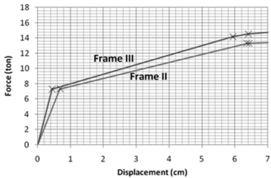
Fig. 10 Comparison between pushover analysis result of Frames II and III
