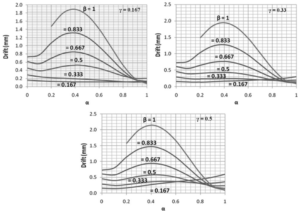
Fig. 3 Modified drifts of wide frames with various value of  $\gamma$
