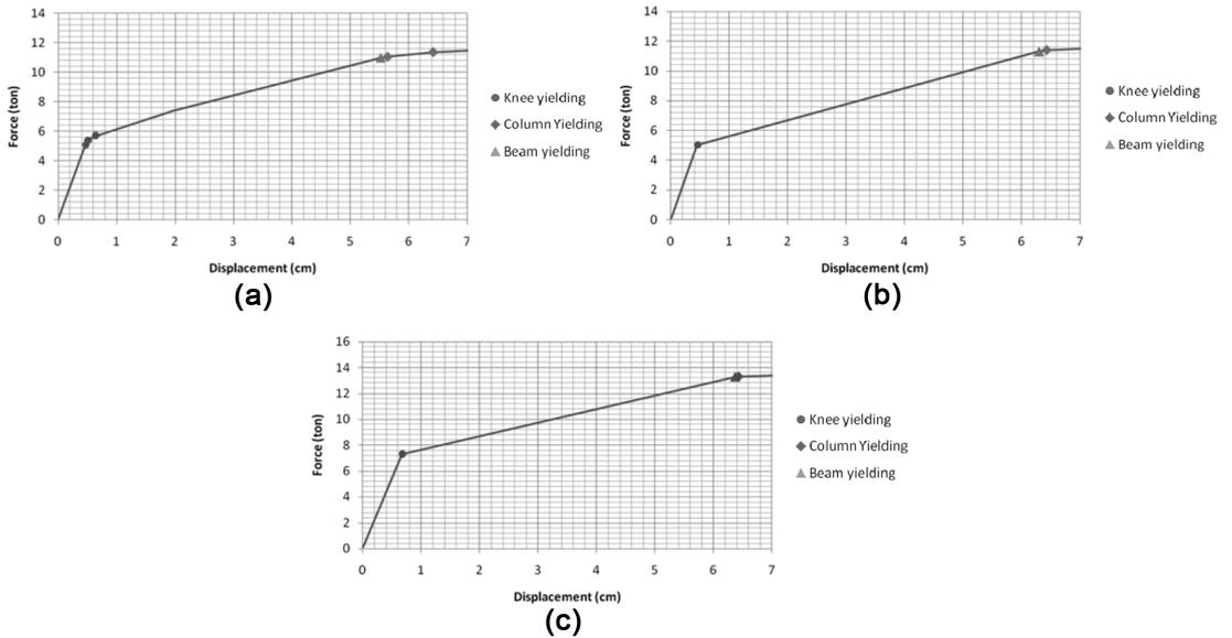
Fig. 7 Load–displacement graph for (a) Base frame, (b) Frame I (c) Frame II
