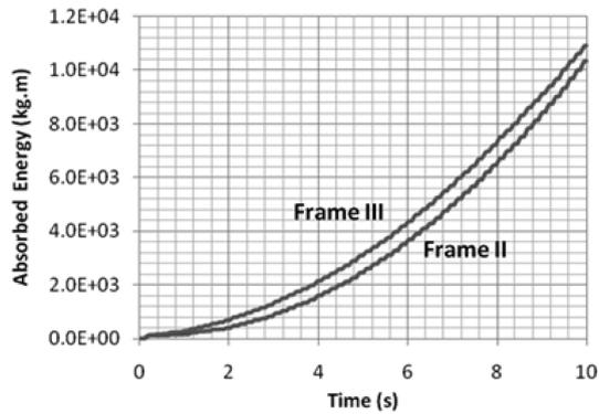
Fig. 11 Comparison between energy dissipation of Frames II and III
