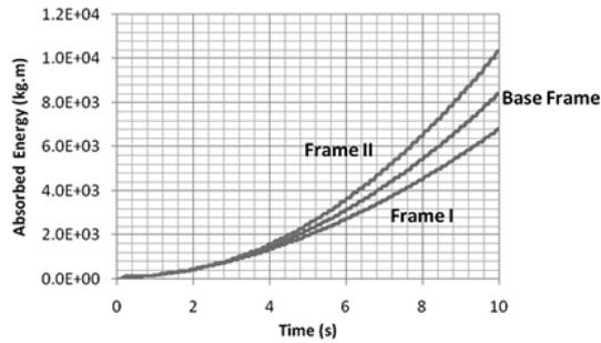
Fig. 9 Cumulative input energy and hysteretic energy dissipation
