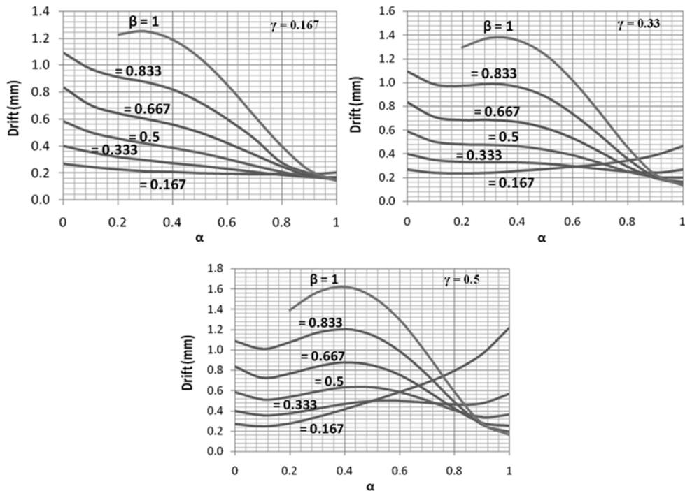
Fig. 4 Modified drift of tall frames with various value of  $\gamma$
