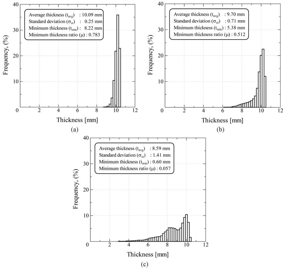
Fig. 5 Thickness histograms of (a) minor corrosion type (F-14), (b) moderate corrosion type (F-13) and (c) severe corrosion type (F-18)
