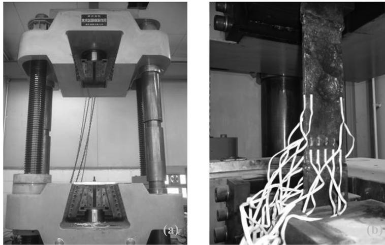
Fig. 6 (a) Loading test machine and (b) specimen prepared for the tensile test
