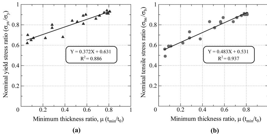
Fig. 9 Relationship of (a) yield stress ratio, (b) tensile stress ratio and minimum thickness ratio ( $\mu$ )
