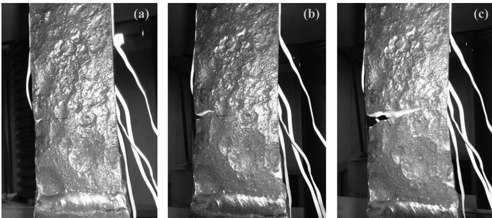
Fig. 8 (a) Crack initiation; (b) and (c) propagation of the crack
