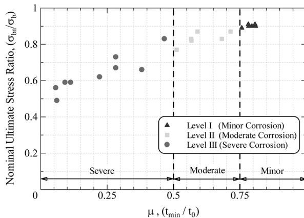
Fig. 3 Relationship of ultimate stress ratio & minimum thickness ratio ( $\mu$ )
