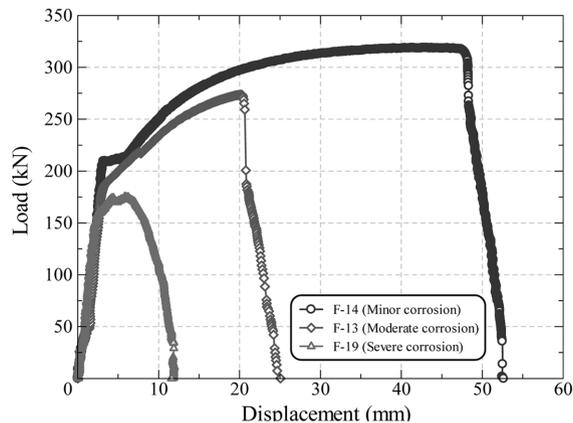
Fig. 7 Load-displacement curves
