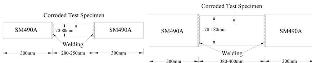
Fig. 1 Dimensions of test specimens
