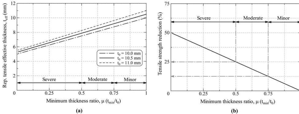
Fig. 12 Relationship of (a) representative tensile effective thickness ( $t_{eff}$ ), (b) tensile strength reduction and minimum thickness ratio ( $\mu$ )
