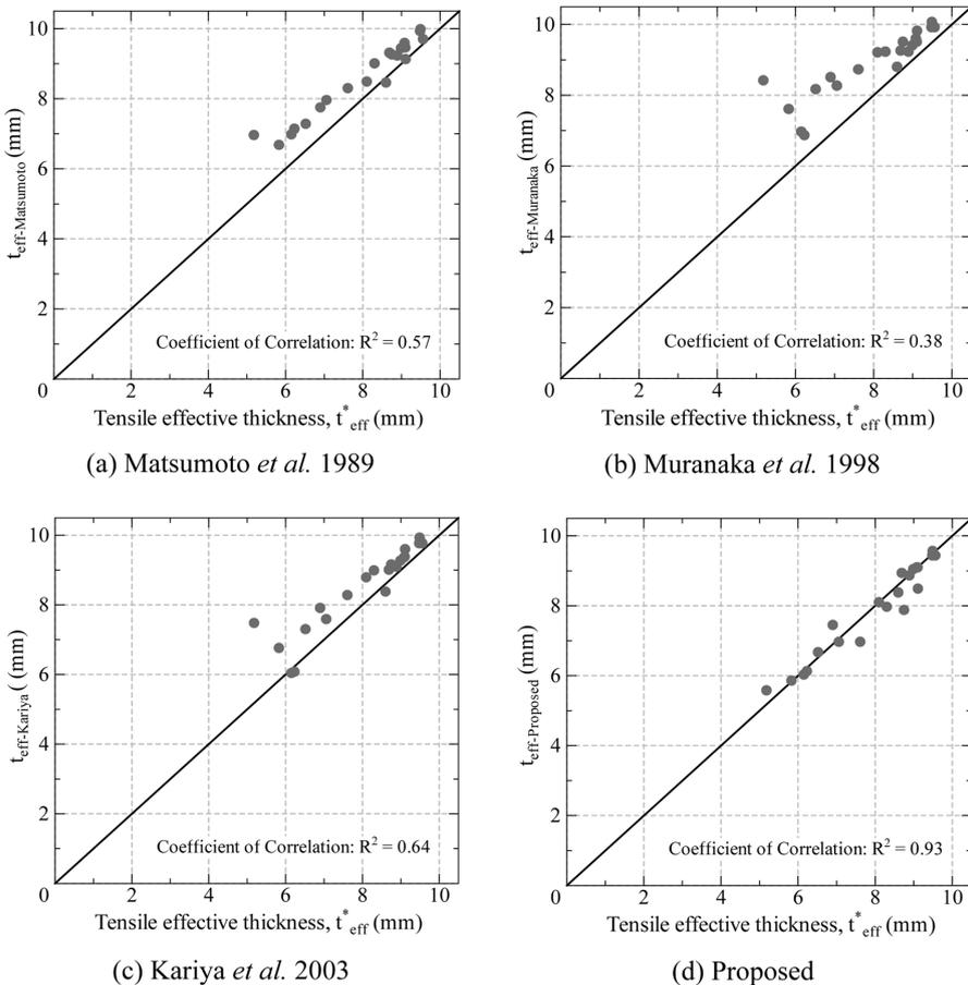
Fig. 11 Relation between different predicted effective thickness parameters with  $t_{eff}^*$
