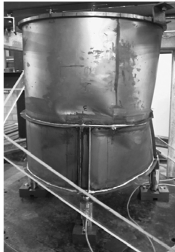
Fig. 1 Buckling mode - failure occurs above the upper ring
