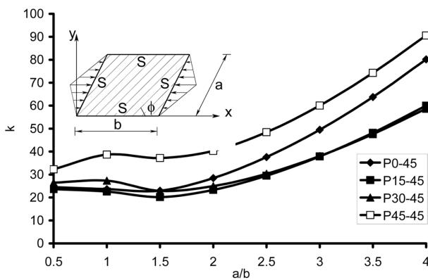
Fig. 12 Variation of  $k$  with aspect ratio for  $\phi = 45^\circ$  (triangular inplane load)
