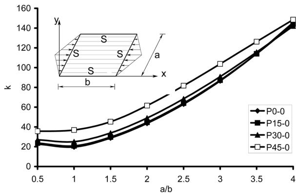
Fig. 10 Variation of  $k$  with aspect ratio for  $\phi = 0^\circ$  (triangular inplane load)
