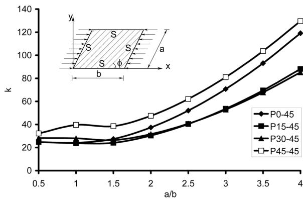
Fig. 7 Variation of  $k$  with aspect ratio for  $\phi = 45^\circ$  (uniform inplane load)
