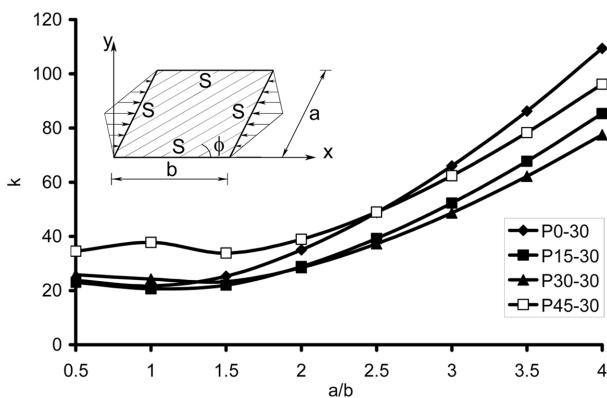
Fig. 11 Variation of  $k$  with aspect ratio for  $\phi = 30^\circ$  (triangular inplane load)
