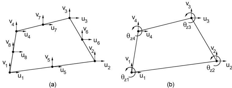
Fig. 2 Displacements for (a) 8-node membrane (b) 4-node membrane
