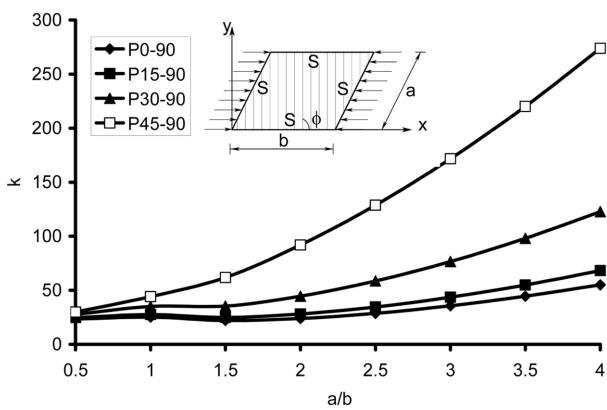
Fig. 9 Variation of  $k$  with aspect ratio for  $\phi = 90^\circ$  (uniform inplane load)
