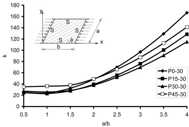
Fig. 6 Variation of  $k$  with aspect ratio for  $\phi = 30^\circ$  (uniform inplane load)
