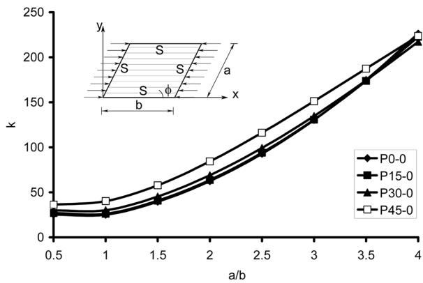
Fig. 5 Variation of  $k$  with aspect ratio for  $\phi = 0^\circ$  (uniform inplane load)
