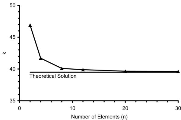
Fig. 4 Convergence of  $k$  with number of elements for a square isotropic plate
