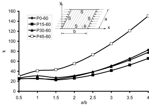
Fig. 8 Variation of  $k$  with aspect ratio for  $\phi = 60^\circ$  (uniform inplane load)
