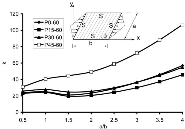
Fig. 13 Variation of  $k$  with aspect ratio for  $\phi = 60^\circ$  (triangular inplane load)
