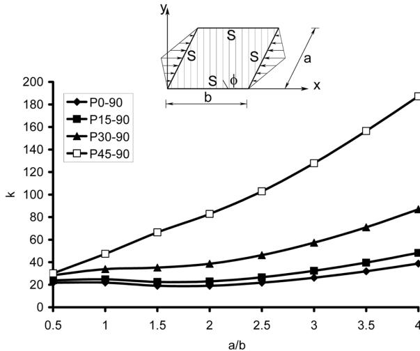
Fig. 14 Variation of  $k$  with aspect ratio for  $\phi = 90^\circ$  (triangular inplane load)
