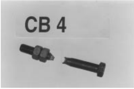
Fig. 12 Failed bolt from CB4 test
