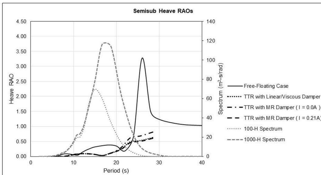
Fig. 7 Input wave spectra and heave RAOs for free-floating and with TTR+dampers cases
