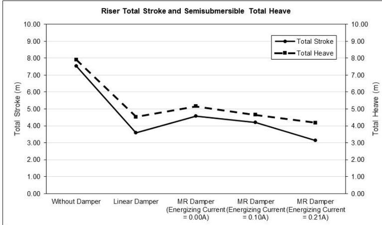
Fig. 12 Riser total stroke (TTR2) and semisubmersible total heave
