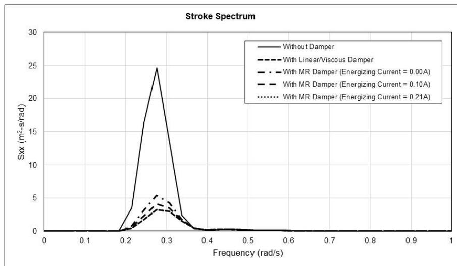
Fig. 9 Riser-stroke (TTR2) spectra
