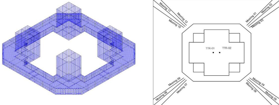
Fig. 6 Isometric view and top view of the semisubmersible
