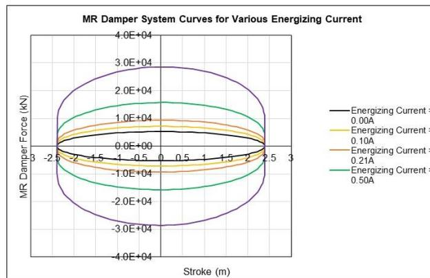
Fig. 3 MR damper stiffness (force versus stroke) curve for various energizing current
