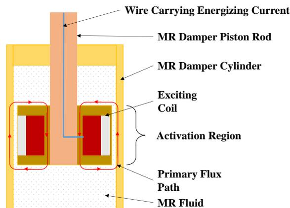
Fig. 1 Schematic and configuration of an MR damper
