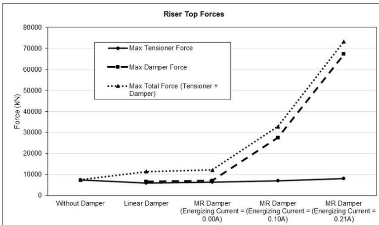
Fig. 13 Riser-top forces (Tensioner w/wo dampers)
