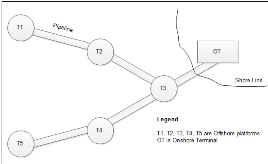
Fig. 1 Layout of the shallow water offshore-onshore gas field complex
