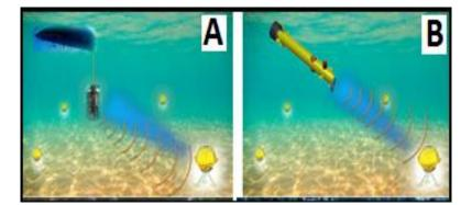
Fig. 1 Rendering showing OWC in data collection from an offshore node
