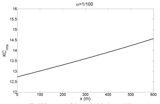
Fig. 5 *KC*<sub>rms</sub> versus x in finite water depth for slope  $\alpha = 1/100$
