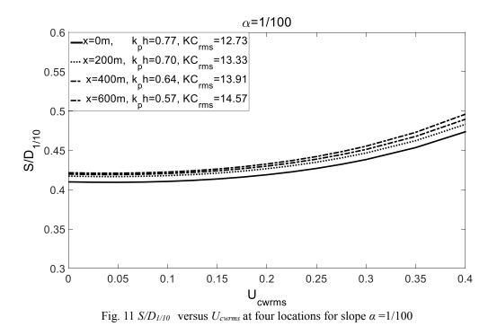
Here the alternative view of the scour process is considered using the results of the present stochastic method. The question is how well the mean scour depth caused by the  $(1/n)^{\text{th}}$  highest waves,  $E[S(H)|H > H_{1/n}]$  (see Eq. (47)), can be represented by using the mean of the  $(1/n)^{\text{th}}$  highest waves in the scour depth formula for regular waves, i.e.,  $S(E[H_{1/n}])$ .
