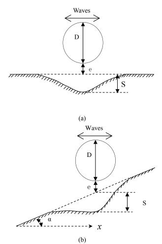
Fig. 14 Definition sketch of scour below pipelines with a pipe position e above the undisturbed bed: (a) on a horizontal bed; (b) on a mild slope
