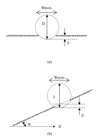
Fig. 15 Definition sketch of self-burial depth B at span shoulder of pipelines: (a) on a horizontal bed; (b) on a mild slope
