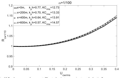
Fig. 13 Random waves plus current: The stochastic to approximate method ratio  $R_{cw1/10}$  versus  $U_{cwrms}$  at four locations for slope  $\alpha = 1/100$
