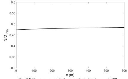
Fig. 7 *S*/ $D_{1/10}$  versus *x* in finite water depth for slope  $\alpha = 1/100$
