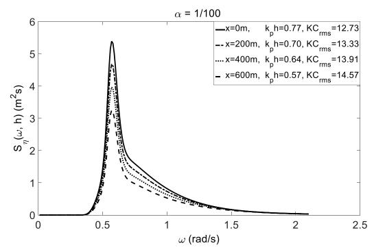
Fig. 4 The transitional wave spectra in finite water depth  $S_{\eta}(\omega, h)$  versus  $\omega$  at four locations for slope  $\alpha = 1/100$
