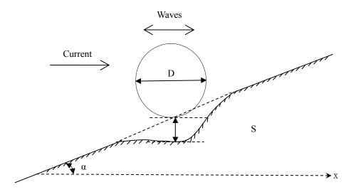
Fig. 2 Definition sketch of the scour depth (S) below a pipeline with diameter (D) on a mild slope ( $\alpha$ )
