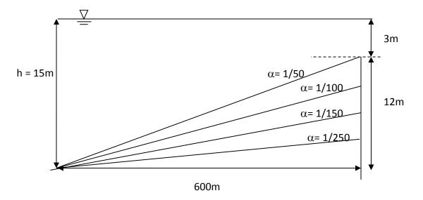
Fig. 8 Sketch of the seabed conditions for four slopes  $\alpha = (1/50, 1/100, 1/150, 1/250)$ . The total horizontal length of the sloping bed is 600 m, and the water depth at the seaward direction is 15 m
