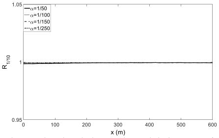
Fig. 12 Random waves alone: The stochastic to approximate method ratio  $R_{1/10}$  versus *x* for four slopes  $\alpha = (1/50, 1/100, 1/150, 1/250)$
