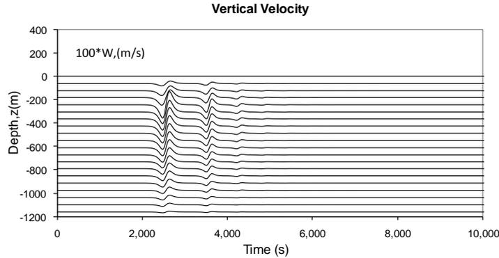
Fig. 5 Vertical Velocity Distribution with Depth ( $\eta=170$  m)
