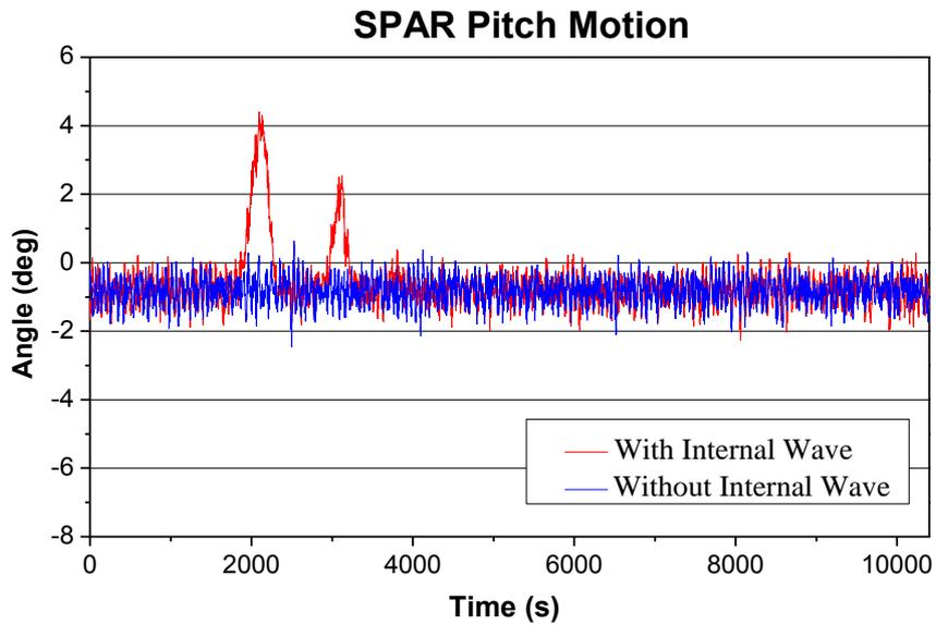
Fig. 13 Spar Pitch Motion Time History ( $\eta=170$  m)
