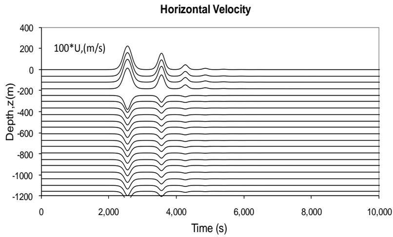
Fig. 4 Horizontal Velocity Distribution with Depth ( $\eta=170$  m)
