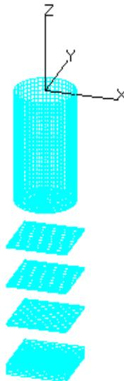
Fig. 9 Panel Model of Spar
