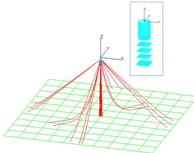
Fig. 10 Spar Coupled Analysis Model with Program HARP
