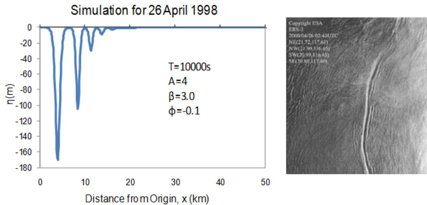
Fig. 2 Internal Wave Model and the Corresponding Satellite Picture (April 26, 1998)
