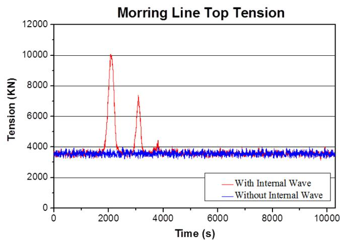
Fig. 14 Spar Mooring Line #5 Top Tension Time History ( $\eta=170$  m)
