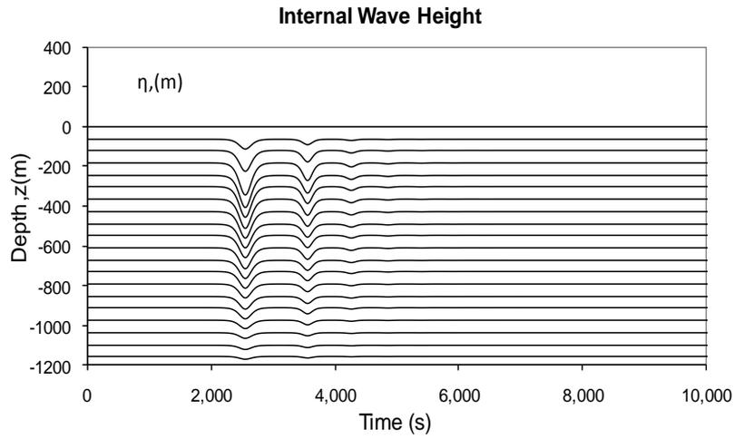
Fig. 3 Internal Wave Height Distribution with Depth ( $\eta=170$  m)
