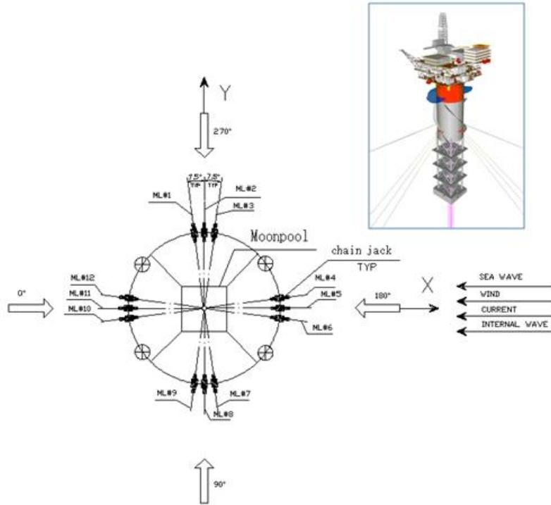
Fig. 8 Spar Configuration and Mooring Layout
