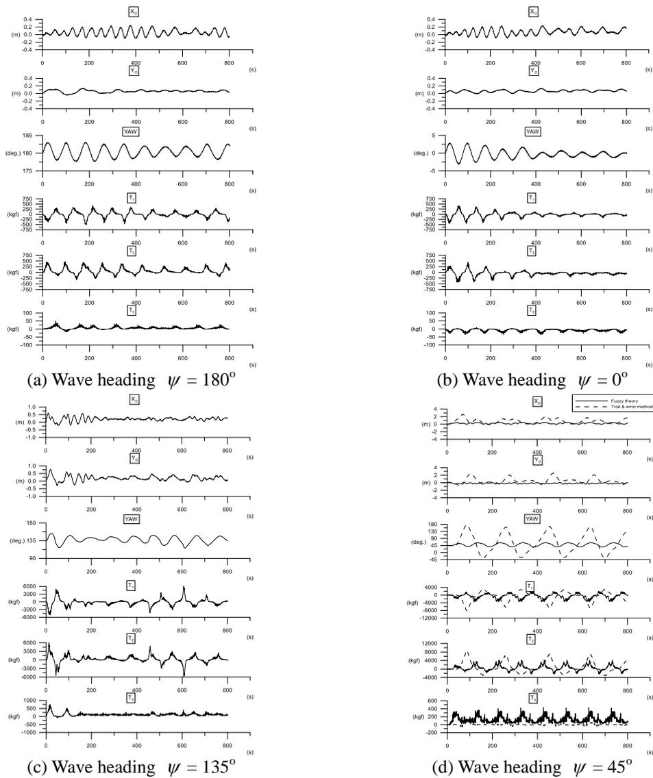
Fig. 4 Time history of the ship horizontal motions and thrust forces with respect to the different dominate wave headings
