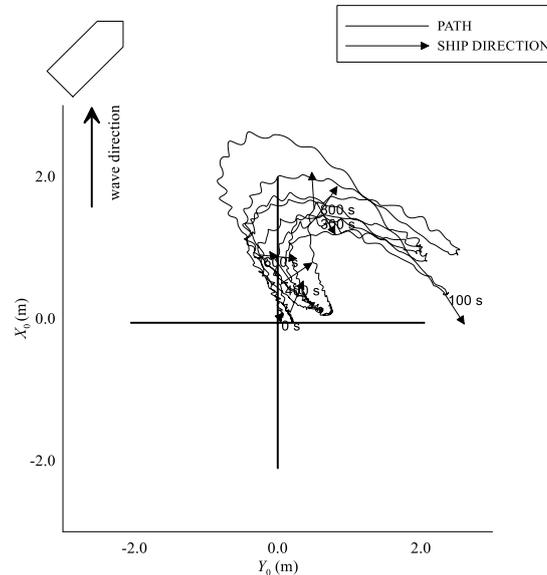
Fig. 8 Ship DP trajectory in  $\psi = 45^\circ$  under DP system, which the control gains of PD control determined by the traditional trial and error method
