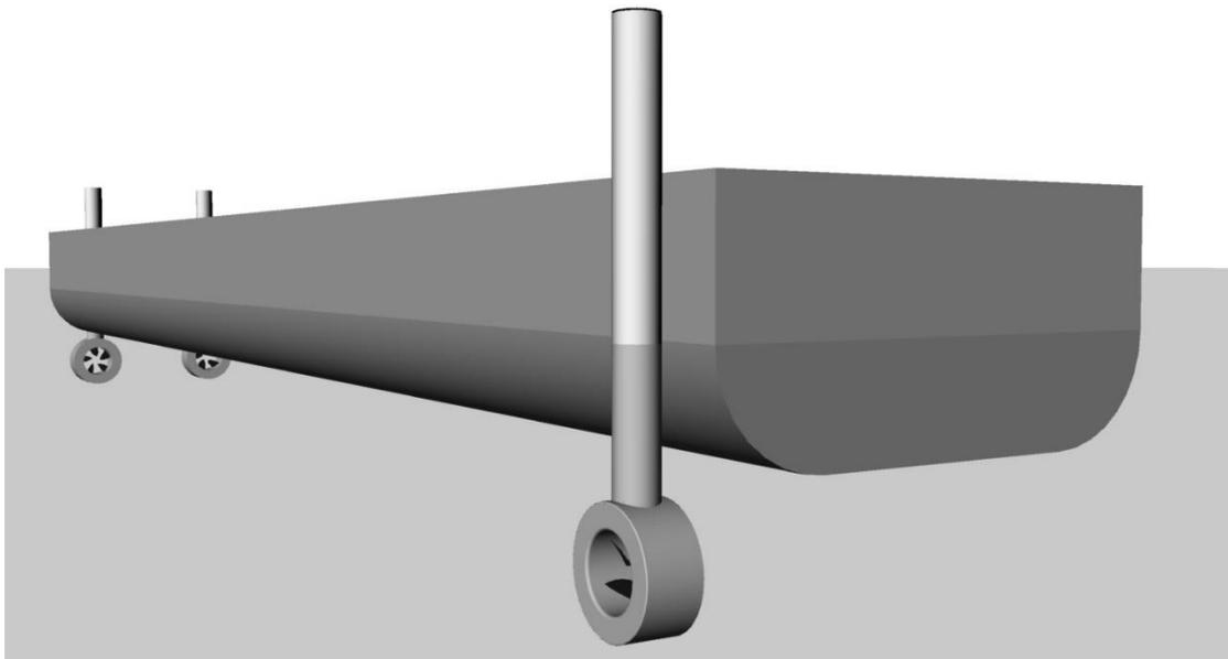
Fig. 3 Arrangement of the three portable outboard thrusters
