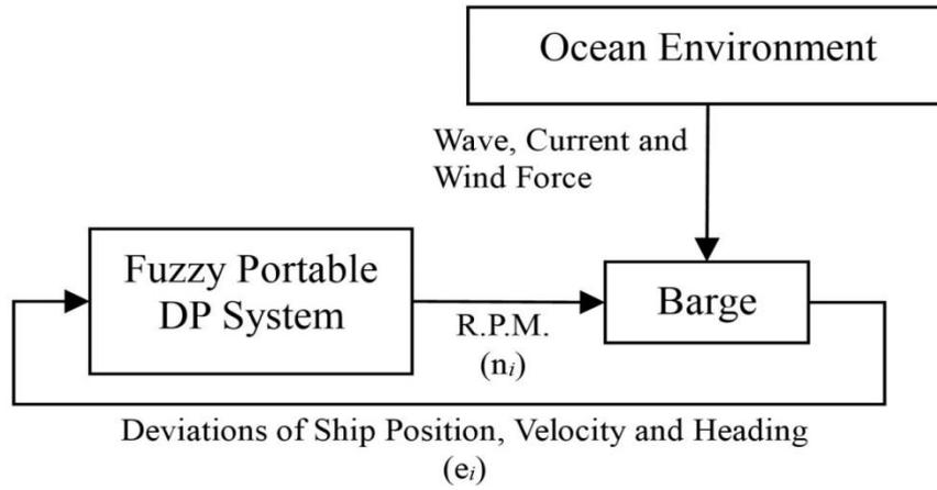
Fig. 2 Control loop of the DP system on the barge
