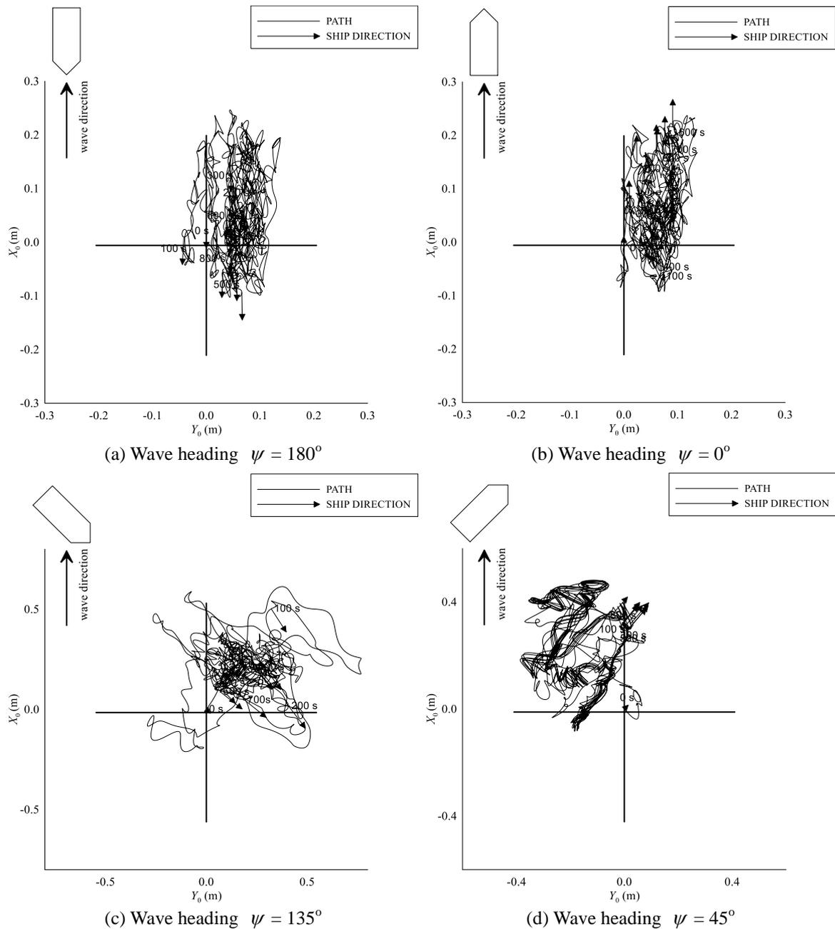
Fig. 7 Ship DP trajectories under DP system, which the R.P.M. of thrusters determined by the present fuzzy algorithm
