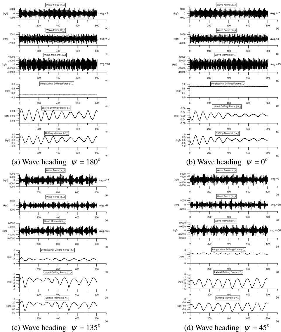
Fig. 5 Time history of the first-order wave forces and drifting forces with respect to the different dominate wave headings
