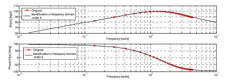
Fig. 2 The identification of the retardation function in frequency domain: the upper one is the amplitude of  $k_z(j\omega)$ ; the lower one is the angle of  $k_z(j\omega)$
