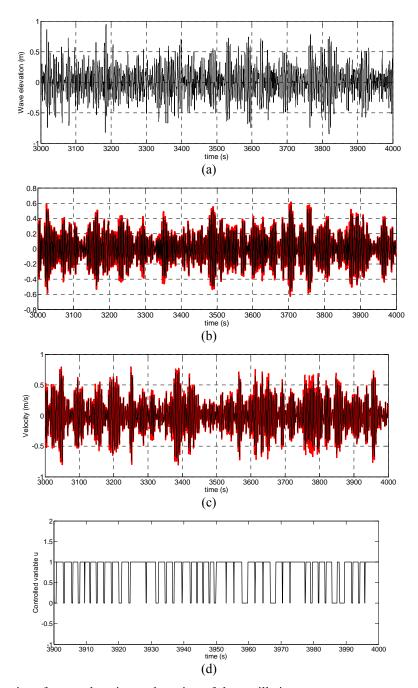
Fig. 10 Time series of wave elevation and motion of the oscillating wave energy converter without and with declutching control based on optimal command method for  $\omega_p = 1.3$  rad/s (red line: motion with declutching control; black line: motion without control): (a) wave elevation; (b) displacement of the converter; (c) velocity of the converter and (d)time sequences of controlled variable u
