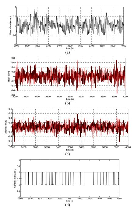
Fig. 9 Time series of wave elevation and motion of the oscillating wave energy converter without and with declutching control based on optimal command method for  $\omega_p = 0.6$  rad/s (red line: motion with declutching control; black line: motion without control): (a) wave elevation (b) displacement of the converter; (c) velocity of the converter and (d)time sequences of controlled variable u
