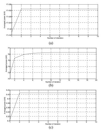
Fig. 4 Absorbed power as a function of the number of iteration with  $A_{\omega}=1$  m  $K=0.1\rho gS$ , C=91000kg/s(a)  $\omega = 0.7rad/s$ ; (b)  $\omega = 1.4rad/s$  and (c)  $\omega = 1.96rad/s$
