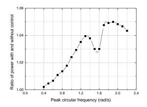
Fig. 8 Ratio of power obtained by the hemispherical wave energy converter without and with declutching control in irregular waves of various peak frequencies
