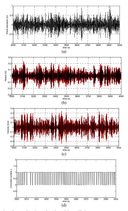
Fig. 11Time series of wave elevation and motion of the oscillating wave energy converter without and with declutching control based on optimal command method for  $\omega_p=2.0$  rad/s (red line: motion with declutching control; black line: motion without control): (a) wave elevation; (b) displacement of the converter; (c) velocity of the converter and (d)time sequences of controlled variable u
