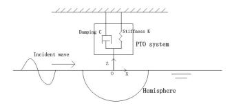
Fig. 1 The sketch of a hemispherical oscillating wave energy converter
