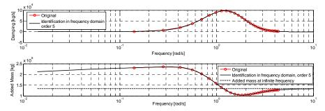
Fig. 3 The identification results of the added mass and radiation damping in frequency domain: the upper one is the radiation damping; the lower one is the added mass
