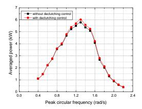
Fig. 7 Power obtained by the hemispherical wave energy converter without and with declutching control in irregular waves of various peak frequencies
