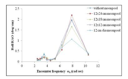
Fig. 11 Roll RAO for different shapes of the moonpool for 3 cm wave height
