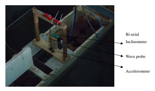
Fig. 7 Ship model with instruments for measurement
