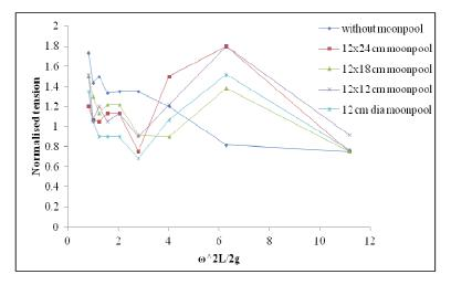
Fig. 13 Mooring line normalized tension for head on side
