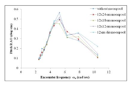
Fig. 12 Pitch RAO with different moonpool shapes for 3cm wave height
