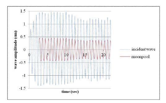
Fig. 9 Incident wave and moonpool water column oscillation for 3cm wave height
