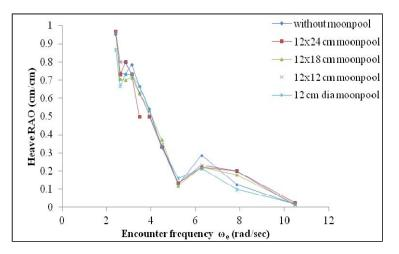
Fig. 10 Heave RAO for different shapes of the moonpool for 3 cm wave height
