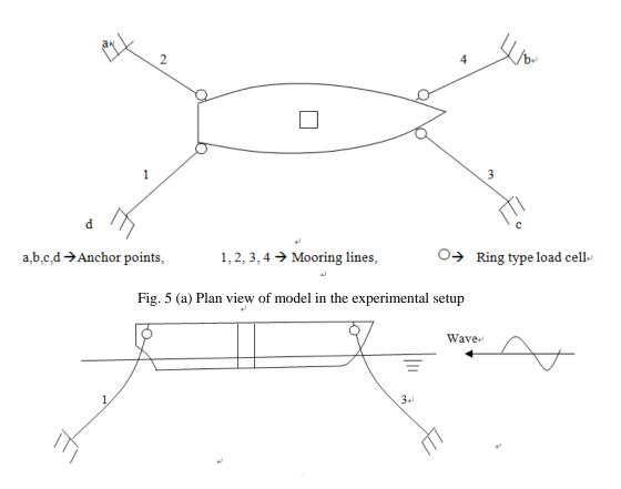
Fig. 5 (b) Schematic sketch of the experimental set up
