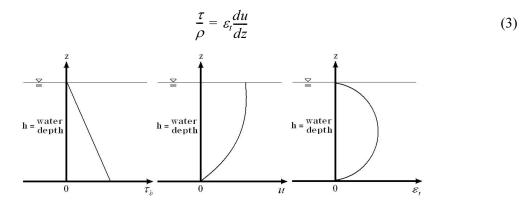
Fig. 1 Vertical distribution of shear stress, velocity, and fluid diffusion coefficient in water column
