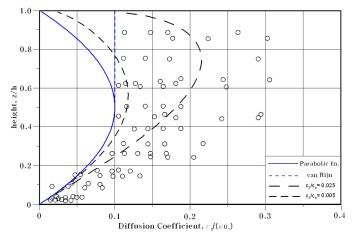
Fig. 6 Composition of computed and measures sediment diffusion coefficient ( $w_f / (\kappa u_*) = 0.758$ )
