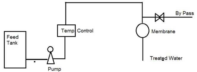
Fig. 1 Membrane pilot schematic
