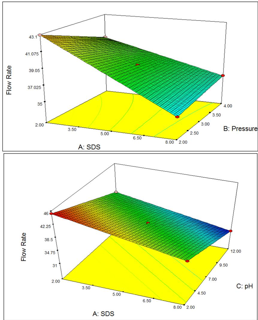
Fig. 5 Influence of pH, SDS and pressure on Flow rate
