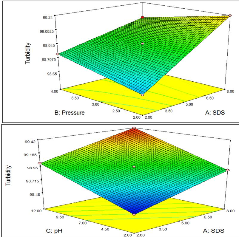
Fig. 2 Influence of pH, SDS and pressure on turbidity
