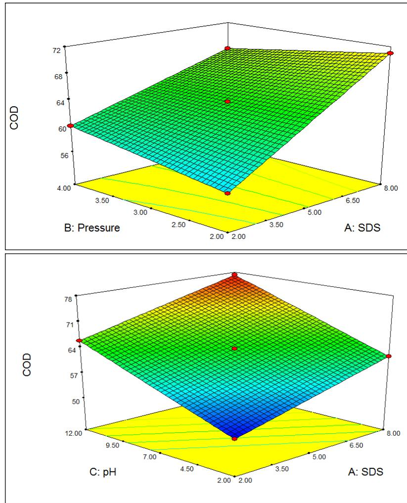
Fig. 4 Influence of pH, SDS and pressure on COD
