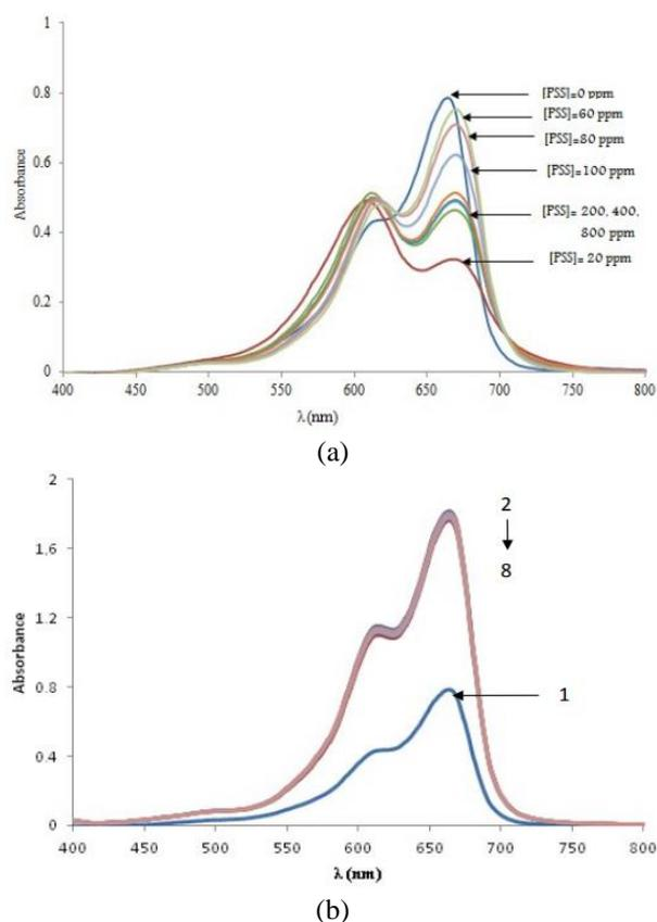
Fig. 3 The visible absorption spectra of MB at 10 ppm in the presence of (a) PSS and (b) PVA at various concentrations (ppm) (1):0, (2):20, (3):60, (4):80, (5):100, (6):200,(7):400 and (8): 800
