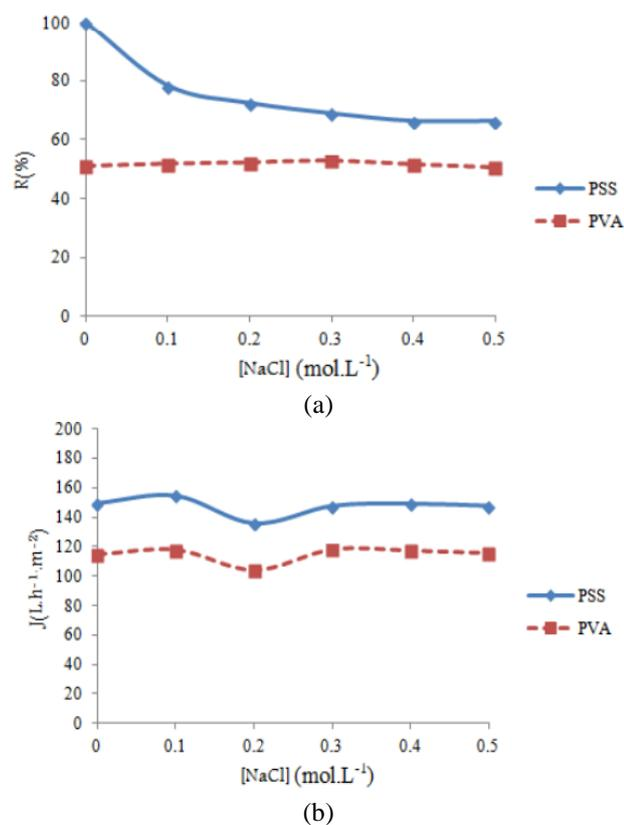
Fig. 7 Effect of NaCl concentration on (a) MB retention and (b) permeate flux at polyelectrolyte concentration of 300 ppm. Feed MB concentration is 100 ppm
