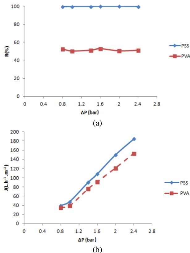
Fig. 6 Effect of transmembrane pressure on (a) MB retention and (b) permeate flux of MB at polyelectrolyte concentration of 300 ppm
