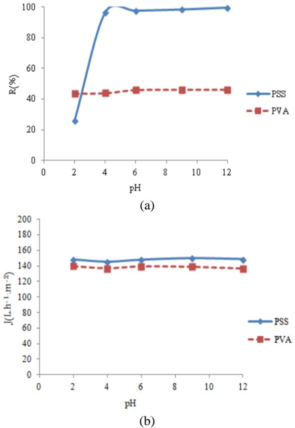
Fig. 8 Effect of pH on (a) MB retention and (b) permeate flux. Concentrations of MB and polyelectrolytes are 100 and 300 ppm, respectively
