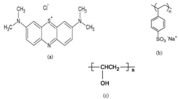
Fig. 1 Molecular structure of (a) methylene blue, (b) poly(sodium 4-styrenesulfonate) and (c) poly(vinyl alcohol)
