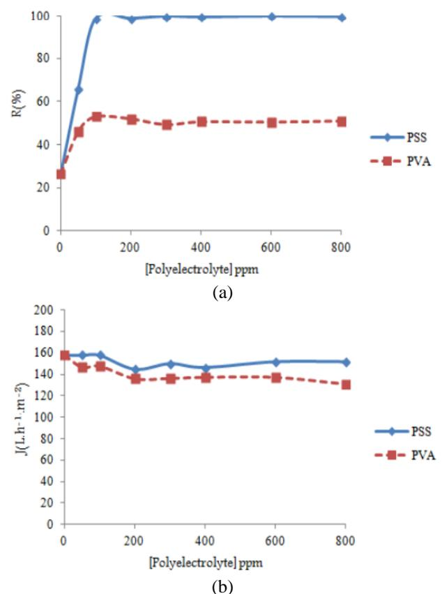
Fig. 5 Variation of (a) MB retention and (b) permeate flux as a function of feed polyelectrolyte concentration. Feed MB concentration is 100 ppm
