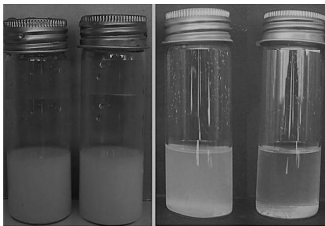
Fig. 8 Sedimentation test (a) just after sonication; (b) after 12 h: the left tube is TiO<sub>2</sub> in mixed solvent-PEG and the right is in DMAc
