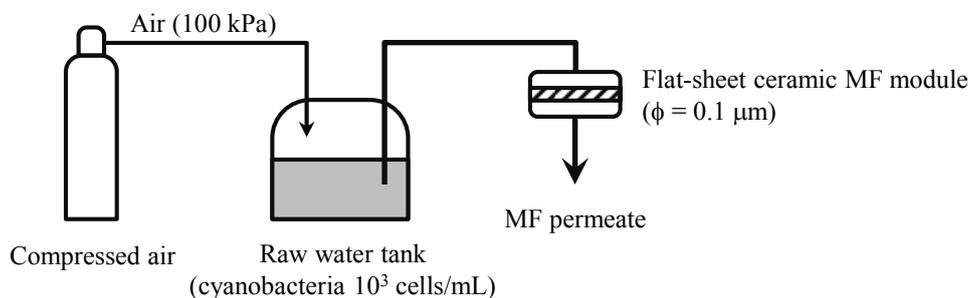
Fig. 1 Experimental setup for laboratory-scale MF experiments
