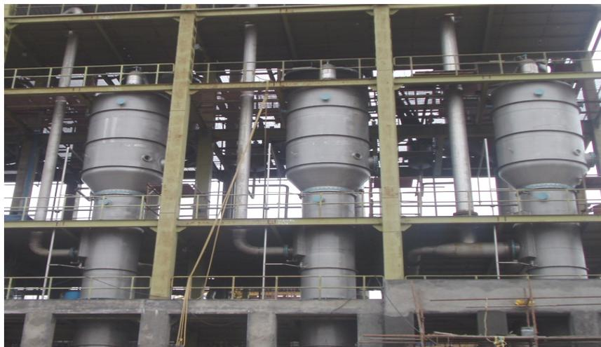
Fig. 5 Site photo showing “Multi Effect Evaporator using TVR”
