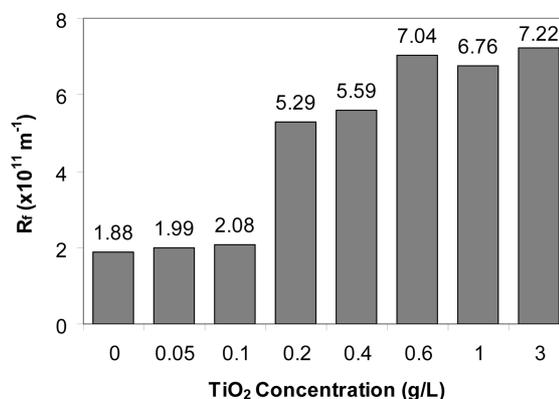
Fig. 7 Effect of TiO<sub>2</sub> concentration on fouling resistance (R<sub>f</sub>); membrane = 0.22 μm PP, [TOC]<sub>0</sub> = 10 mg/L, HA solution filtered for 150 min
