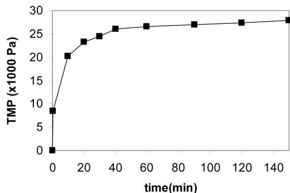
Fig. 3 Characteristic TMP profile of SMPR experiments;  $[\text{TOC}]_0 = 10 \text{ mg/L}$ ,  $\text{TMP}_0 = 8400 \text{ Pa}$ , membrane =  $0.22 \mu\text{m PP}$ ,  $[\text{TiO}_2] = 0.6 \text{ g/L}$ , feed water = HA model solution
