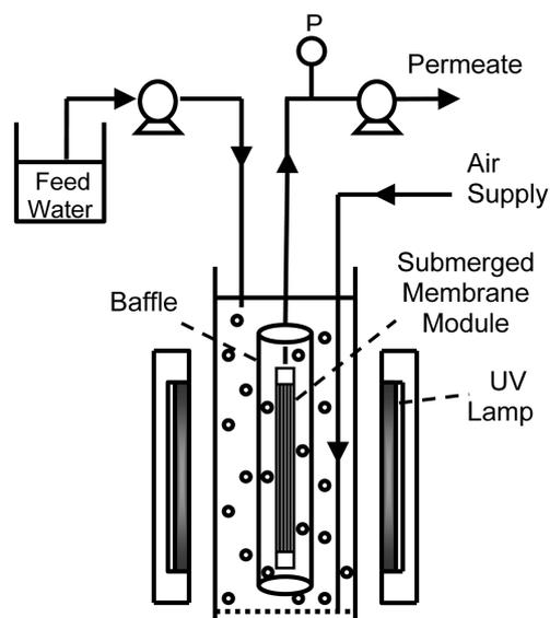
Fig. 1 Schematic of the SMPR experimental setup
