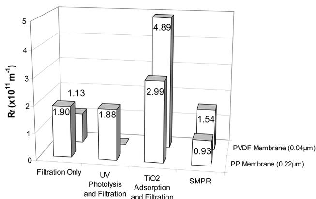
Fig. 5 Relative effect of individual processes on fouling resistance ( $R_f$ );  $[\text{TOC}]_0 = 10 \text{ mg/L}$ , feed water = HA model solution, duration = 60 min. When used,  $[\text{TiO}_2] = 0.5 \text{ g/L}$
