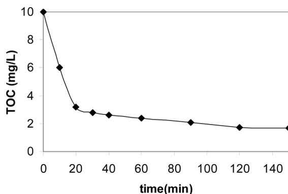
Fig. 2 Characteristic TOC profile of SMPR experiments;  $[\text{TOC}]_0 = 10 \text{ mg/L}$ ,  $\text{TMP}_0 = 8400 \text{ Pa}$ , membrane =  $0.22 \mu\text{m PP}$ ,  $[\text{TiO}_2] = 0.6 \text{ g/L}$ , feed water = HA model solution
