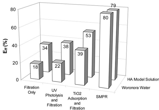
Fig. 9 Effect of pollutant characteristics on organic removal efficiency ( $E_{ff}$ ); membrane = 0.22  $\mu\text{m}$  PP, filtration for 60 min When used,  $[\text{TiO}_2] = 0.5 \text{ g/L}$
