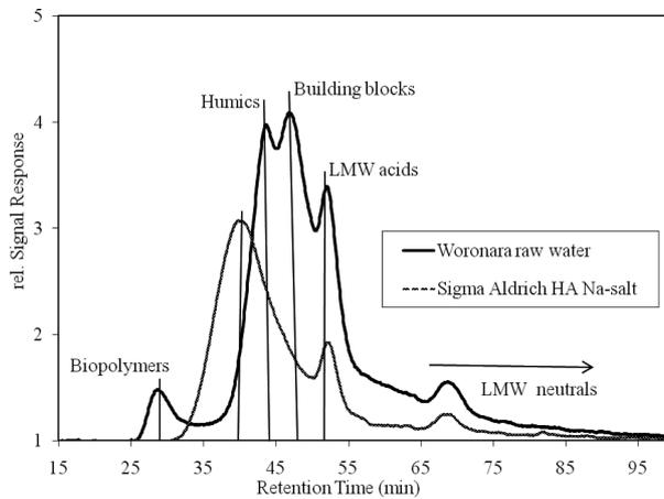
Fig. 8 LC-OCD spectra obtained for Woronara water and synthetic humic acid model solution
