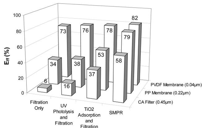
Fig. 4 Relative effect of individual processes on organic removal efficiency ( $E_{ff}$ );  $[\text{TOC}]_0 = 10$  mg/L, feed water = HA model solution, duration = 60 min When used,  $[\text{TiO}_2] = 0.5$  g/L
