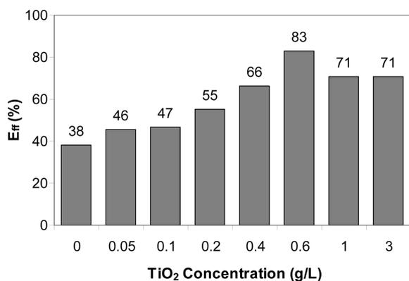
Fig. 6 Effect of TiO<sub>2</sub> concentration on organic removal efficiency (E<sub>eff</sub>); membrane = 0.22 μm PP, [TOC]<sub>0</sub> = 10 mg/L, HA solution filtered for 150 min
