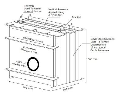
Fig. 2 Test equipment
