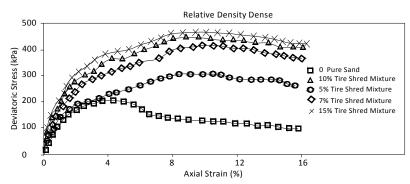
Fig. 7 Axial strain distribution under deviatoric stress
