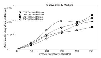
Fig. 14 Maximum bending moment at medium backfill condition
