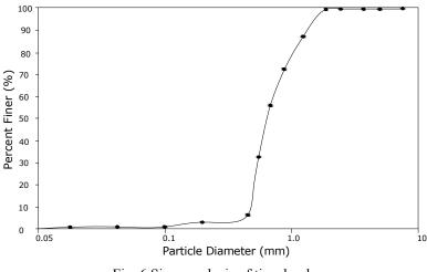
Fig. 6 Sieve analysis of tire shreds
