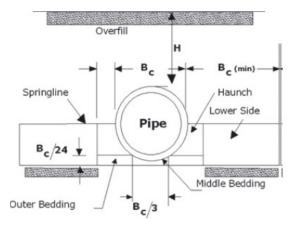
Fig. 1 A Conventional standard trench section (ASTM D 2321)
