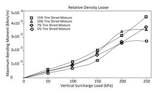
Fig. 13 Maximum bending moment at loose backfill condition
