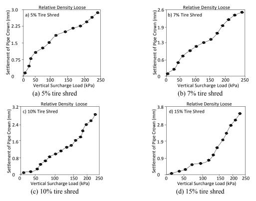
Fig. 10 Vertical deflection of pipe crown in loose backfill condition
