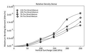
Fig. 15 Maximum bending moment at dense backfill condition
