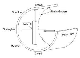
Fig. 3 Section through lined-plain pipe
