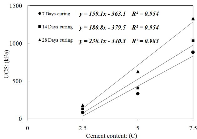
Fig. 7 Effect of cement contents on maximum unconfined compressive strength
