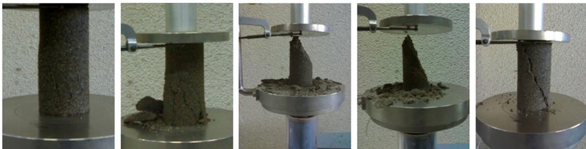
Fig. 10 Failure types of stabilized specimens
