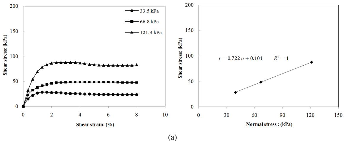
Fig. 11 Effect of cement stabilization on shear stress-strain behavior of soil for 28 curing time in direct shear test associated with Mohr-Coulomb failure envelope: (a) soil without cement; (b) 2.5%; (c) 5%; and (d) 7.5% cement content
