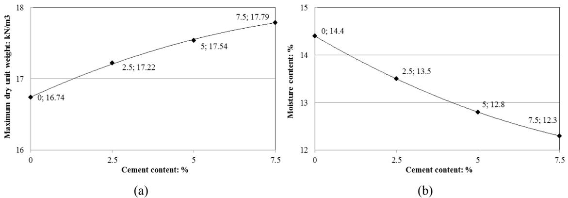
Fig. 4 Effect of cement content on: (a) maximum dry unit weight; and (b) moisture content
