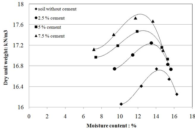
Fig. 3 Effect of cement stabilization on compaction curves
