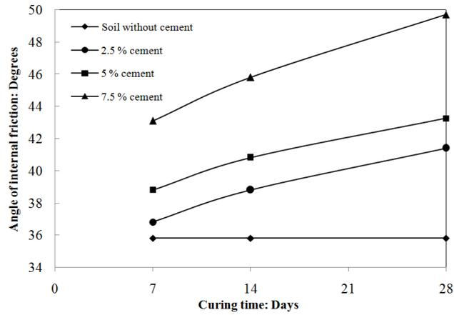
Fig. 12 Shear strength parameters of cement-stabilized soil for different cement content and curing time: (a) cohesion; (b) angle of internal friction
