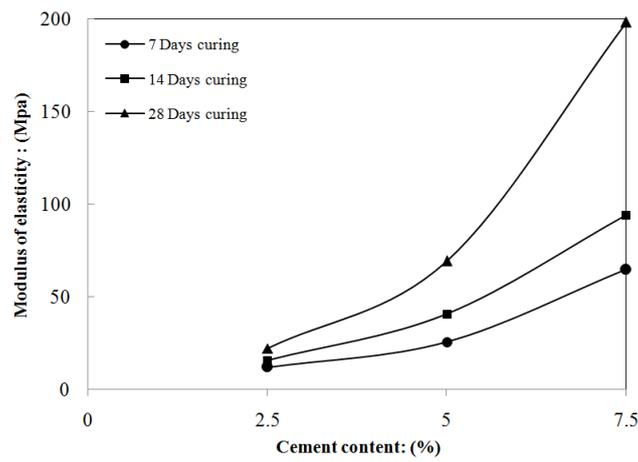
Fig. 9 Effect of cement content and curing time on modulus of elasticity
