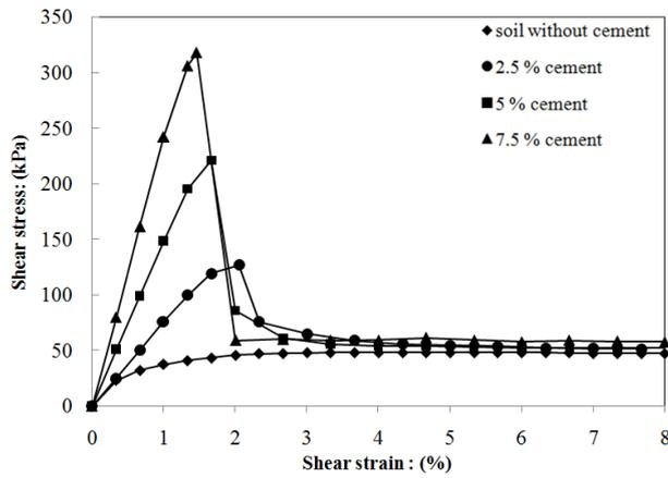
Fig. 13 Stress-strain relationship of cemented and uncemented sandy soils for normal stress of 66.8 kPa
