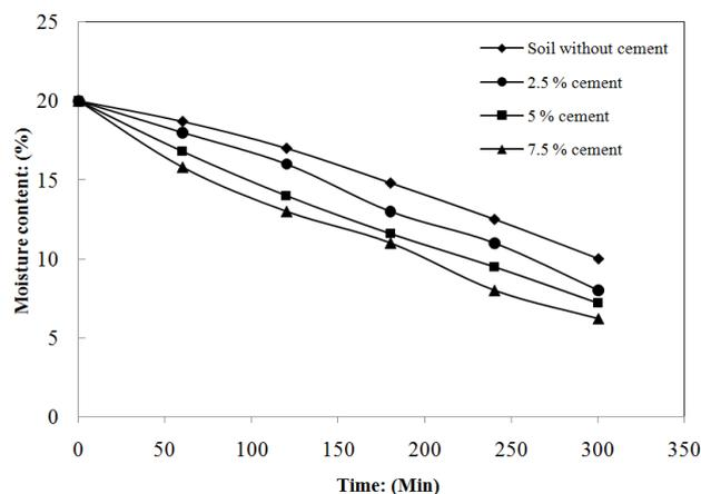
Fig. 5 Solidification characteristics of sandy soil with different cement contents
