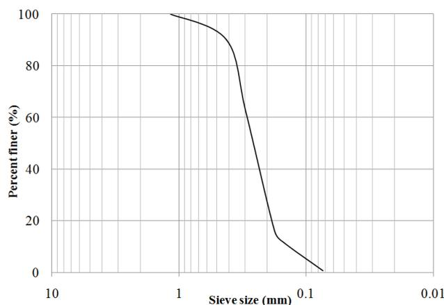
Fig. 1 Grain size distribution curve for Mahmoud-Abad sand
