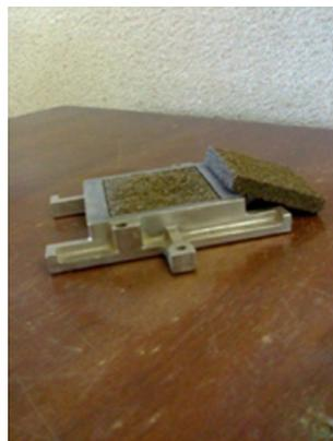
Fig. 14 failure type of stabilized specimen at the end of the direct shear test
