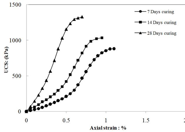
Fig. 8 Effect of curing time on stress-strain behavior for 7.5% cement content
