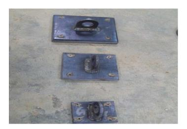
Fig. 4 Symmetrical square anchor plates
