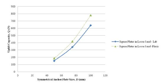
Fig. 8 Variation in uplift capacity Q with square symmetrical anchor plate size D
