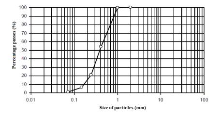
Fig. 2 Particle size distributions for sand sample
