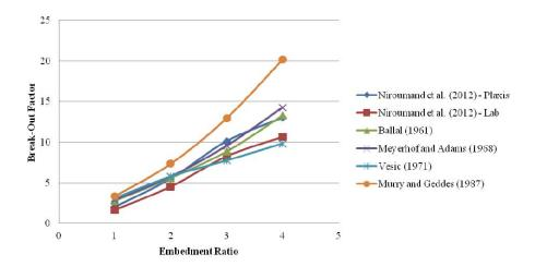
Fig. 13 Comparison of breakout factor between experimental results and theoretical and numerical prediction for square anchor plates in loose packing
