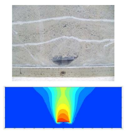
Fig. 12 State of sand after commencement of uplift in loose sand
