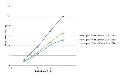
Fig. 10 Variation of breakout factor Nq with embedment ratio L/D for symmetrical square anchor plates in both loose conditions in Plaxis
