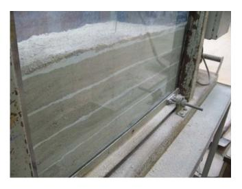
Fig. 11 Initial state of sand before commencement of uplift in loose sand
