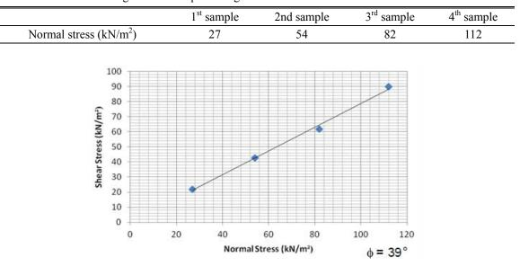
Table 3 Normal stress acting on sand sample during direct shear test
