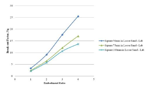
Fig. 9 Variation of breakout factor Nq with embedment ratio L/D for symmetrical square anchor plates in both loose conditions in laboratory
