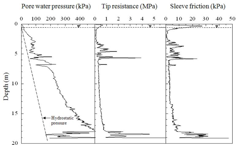
Fig. 8 Piezocone penetration test results at the TB site
