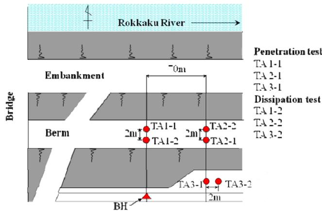
Fig. 3 Plan layout of field tests at TA site (after Chai *et al.* 2004)
