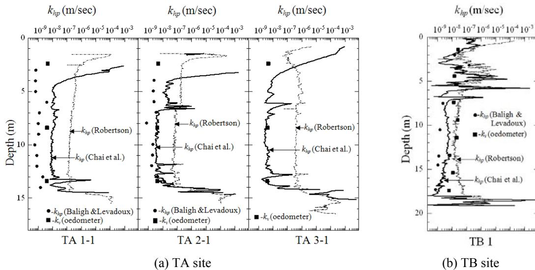
Fig. 12 Hydraulic conductivity from Piezocone test results and laboratory oedometer test results
