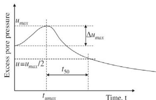
Fig. 1 “Non-standard” dissipation curve
