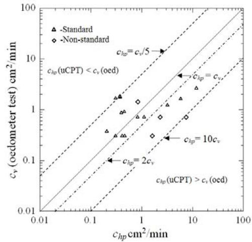
Fig. 11 Comparison of  $c_{hp}$  (uCPT) and  $c_v$  values
