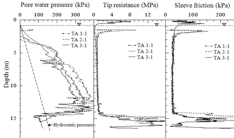
Fig. 5 Piezocone penetration test results at TA site
