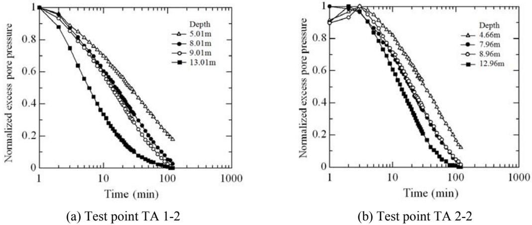
Fig. 6 Dissipation test results at TA site
