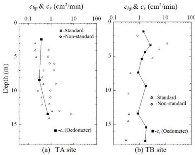
Fig. 10 Test results of  $c_{hp}$  (uCPT) and  $c_v$  (oedometer)
