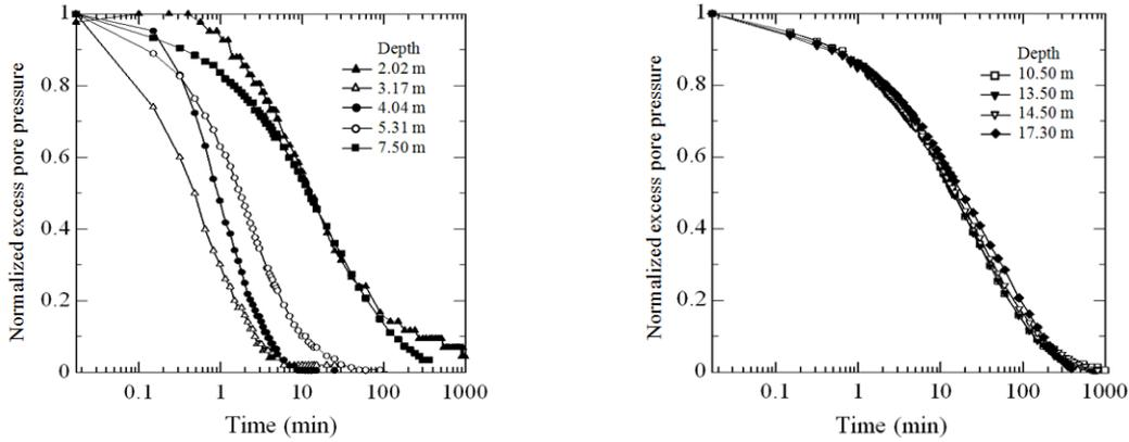
Fig. 9 Field dissipation test results at TB-2
