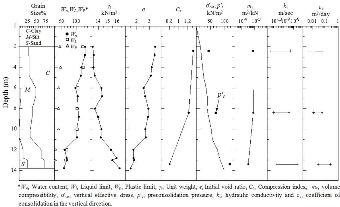
Fig. 4 Some physical and mechanical properties of Ariake clay at the TA site
