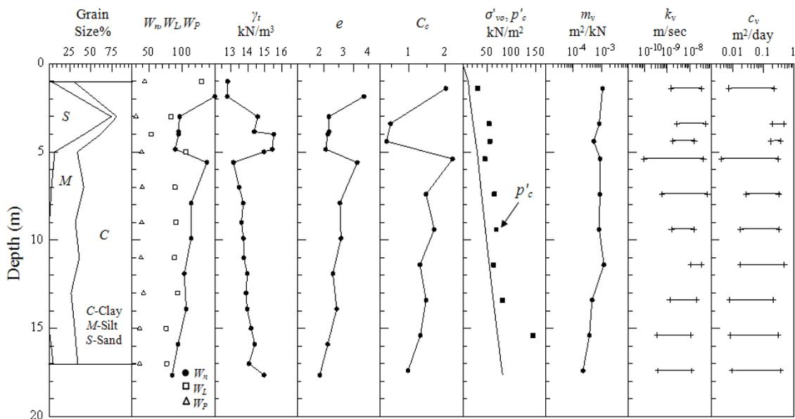
Fig. 7 Some physical and mechanical properties of soils at the TB site
